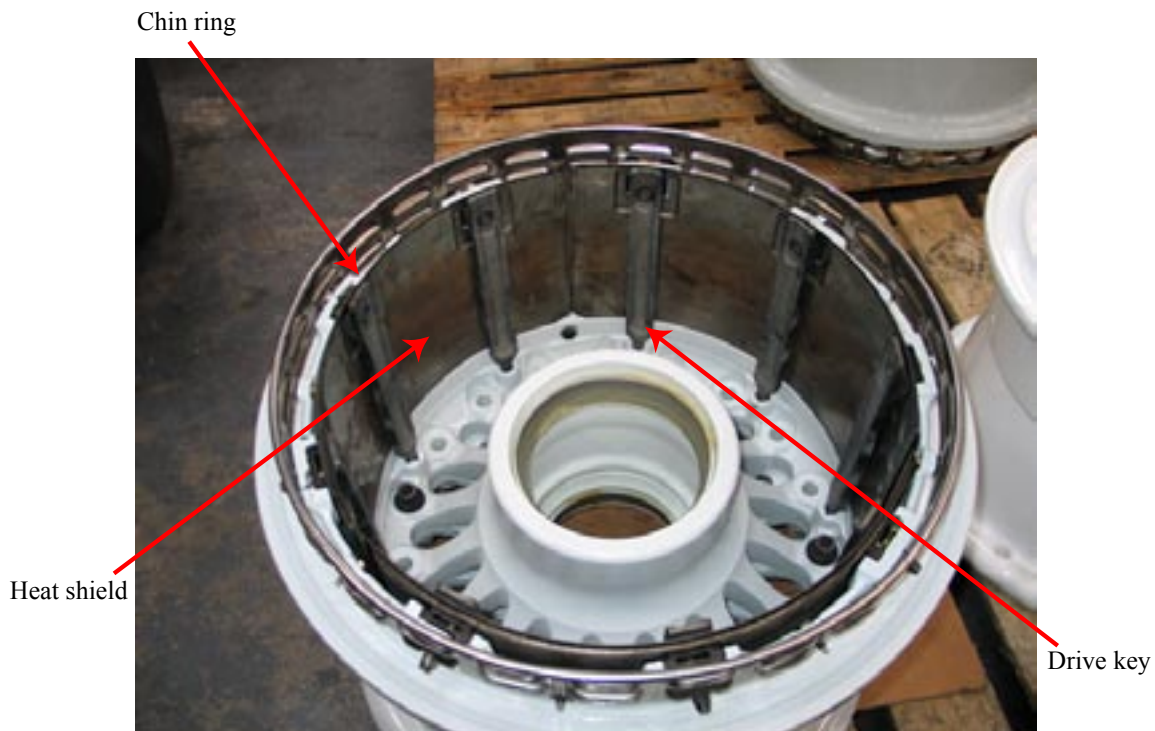
Figure 4 Construction of main wheel
