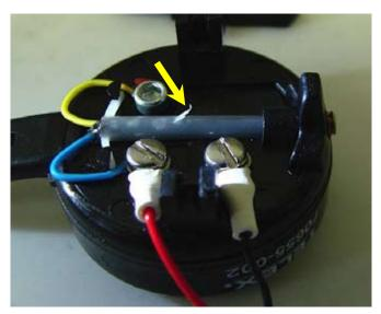
Figure 6 Whisker of plastic material on cut-out switch
