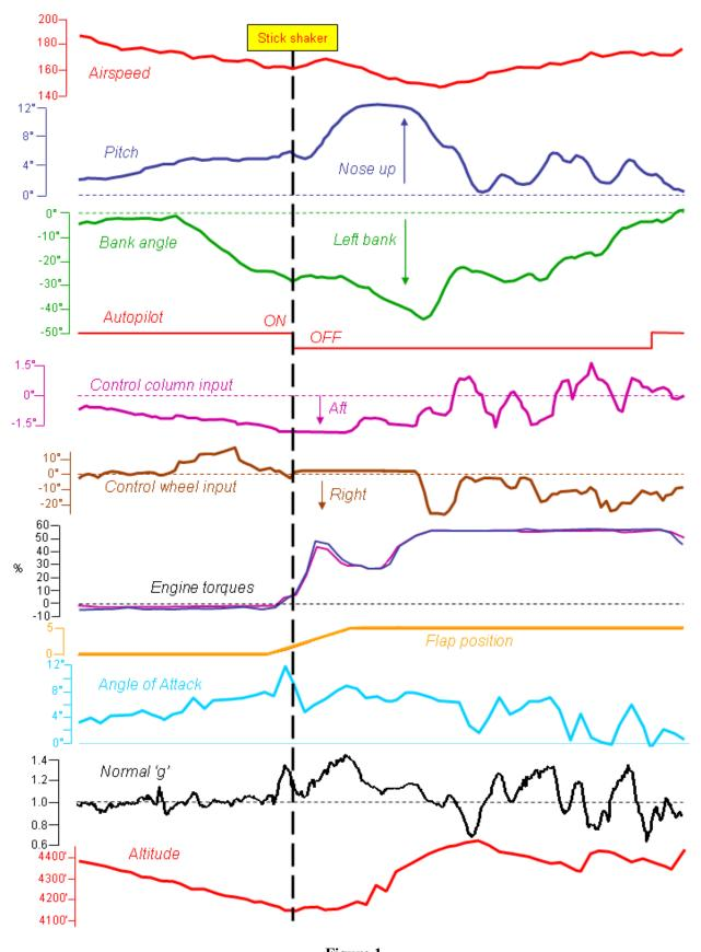
Figure 1 Relevant FDR parameters over a 65 second period surrounding the stick shaker event (simplified)
