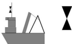
Fishing vessel engaged in fishing displays double cone shape.
