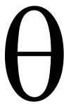
Figure 1 Theta marking for Class 1 radioactive valves. Colour of marking – black. (See Note.)
