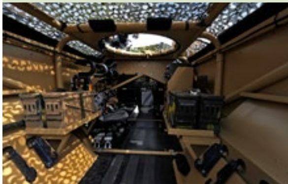
The interior of a Foxhound Light Protected Patrol Vehicle. Foxhound has been specifically designed and built in Britain to protect against the threats faced by troops in Afghanistan. However, this is an agile and versatile vehicle that will be a mainstay in the Army for years to come.
