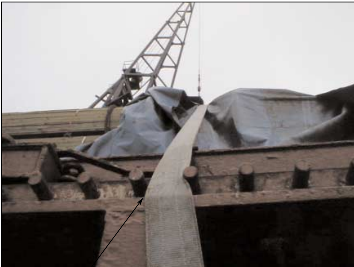
Lashing bent over a relatively sharp hatch cover edge
