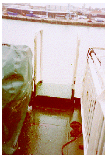
Boarding Bridge in "Open" Position
