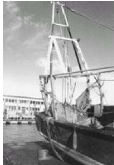
The gantry and A frame
