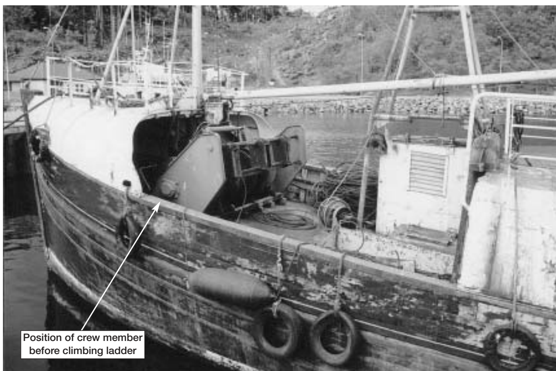
Vessel layout, showing significant freeboard height
