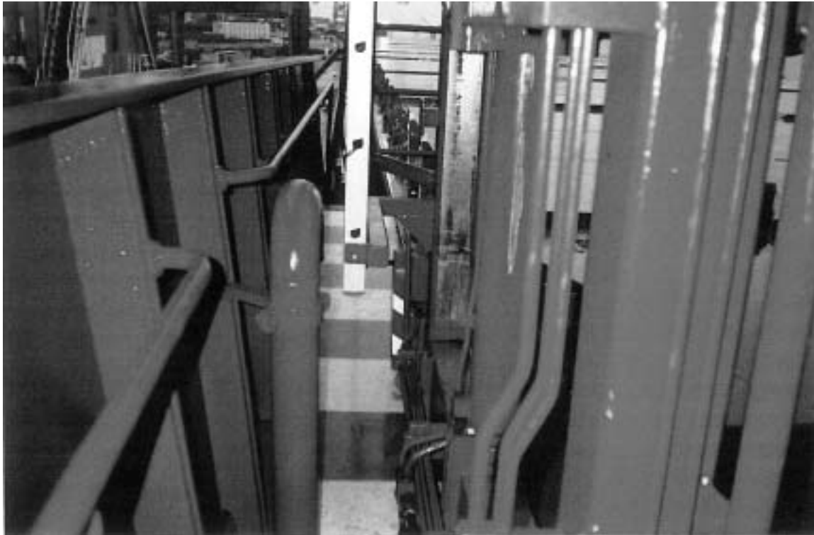
View of walkway from main deck to foc'stle head, showing air vent and hand rails
