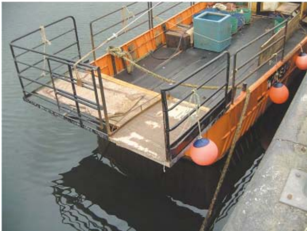
Working deck area showing pound board arrangement
