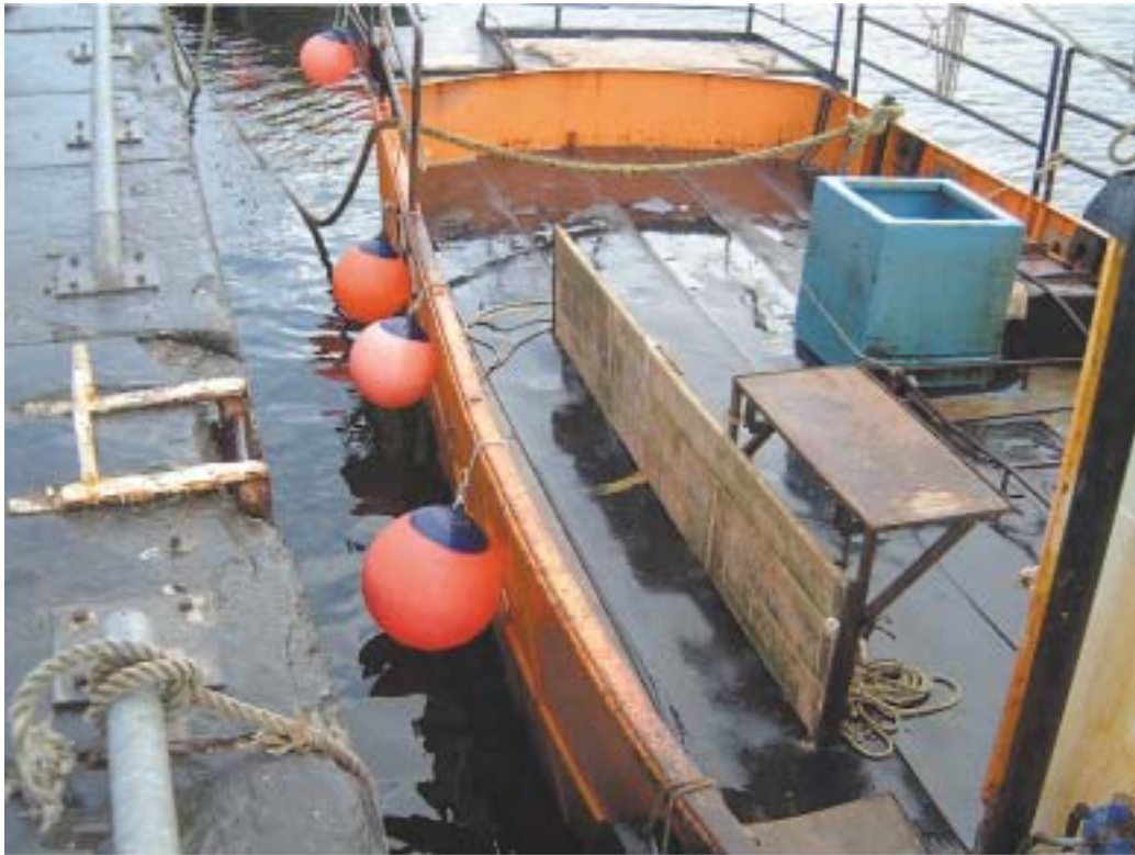
Working deck area showing pound board arrangement
