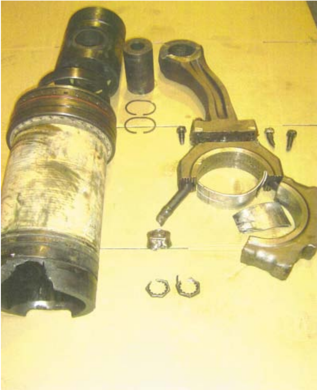
Damage to No 6 Cylinder Components
