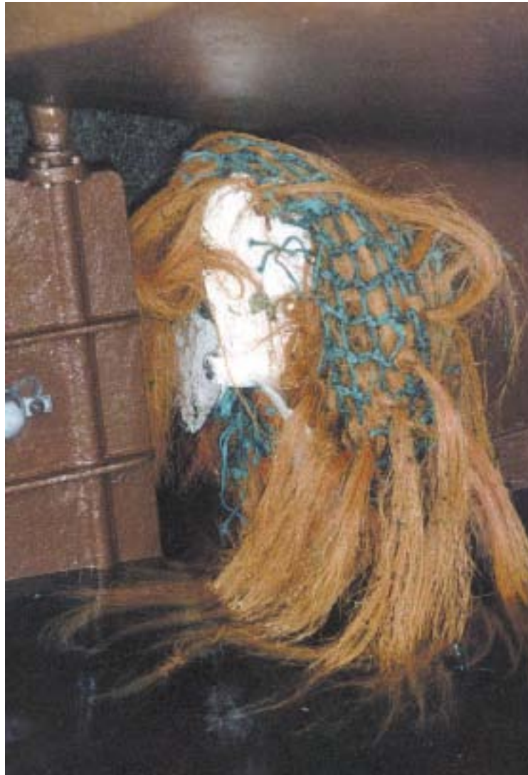
Photograph of propeller fouled by discarded fishing gear
