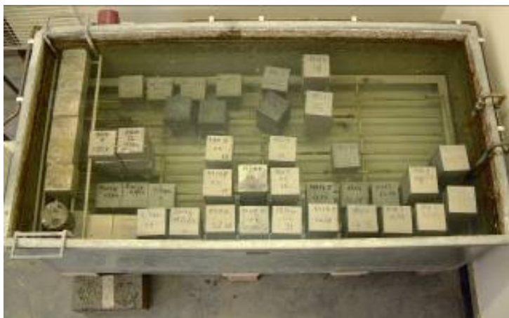
Figure 4 - Laboratory curing and testing of cementitious mixture samples
