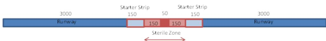
**Figure 4-3 Provision of 150m Starter Strips for Extended Northern Runway**
