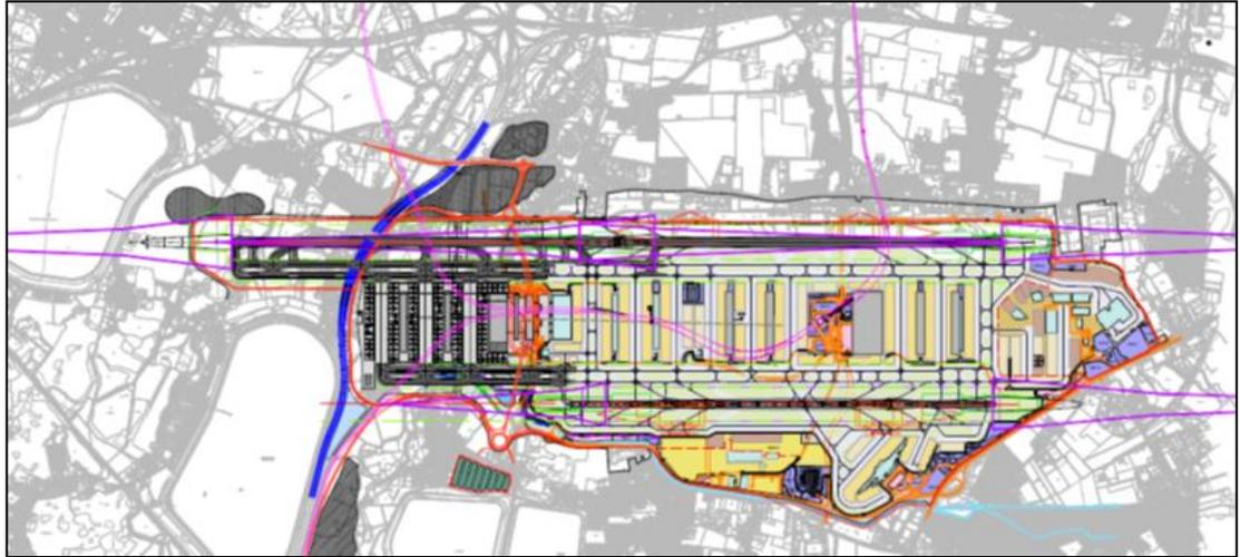
**Figure 4-1 Heathrow Airport Extended Northern Runway Proposed PSZ Contours (Source: Heathrow Hub Ltd submission to the Airports Commission)**
