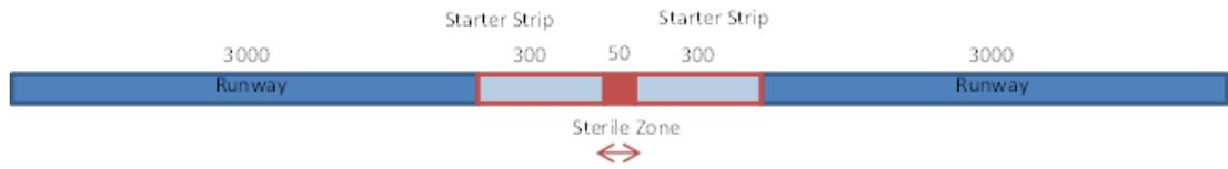
**Figure 4-4 Provision of 300m Starter Strips for Extended Northern Runway**
