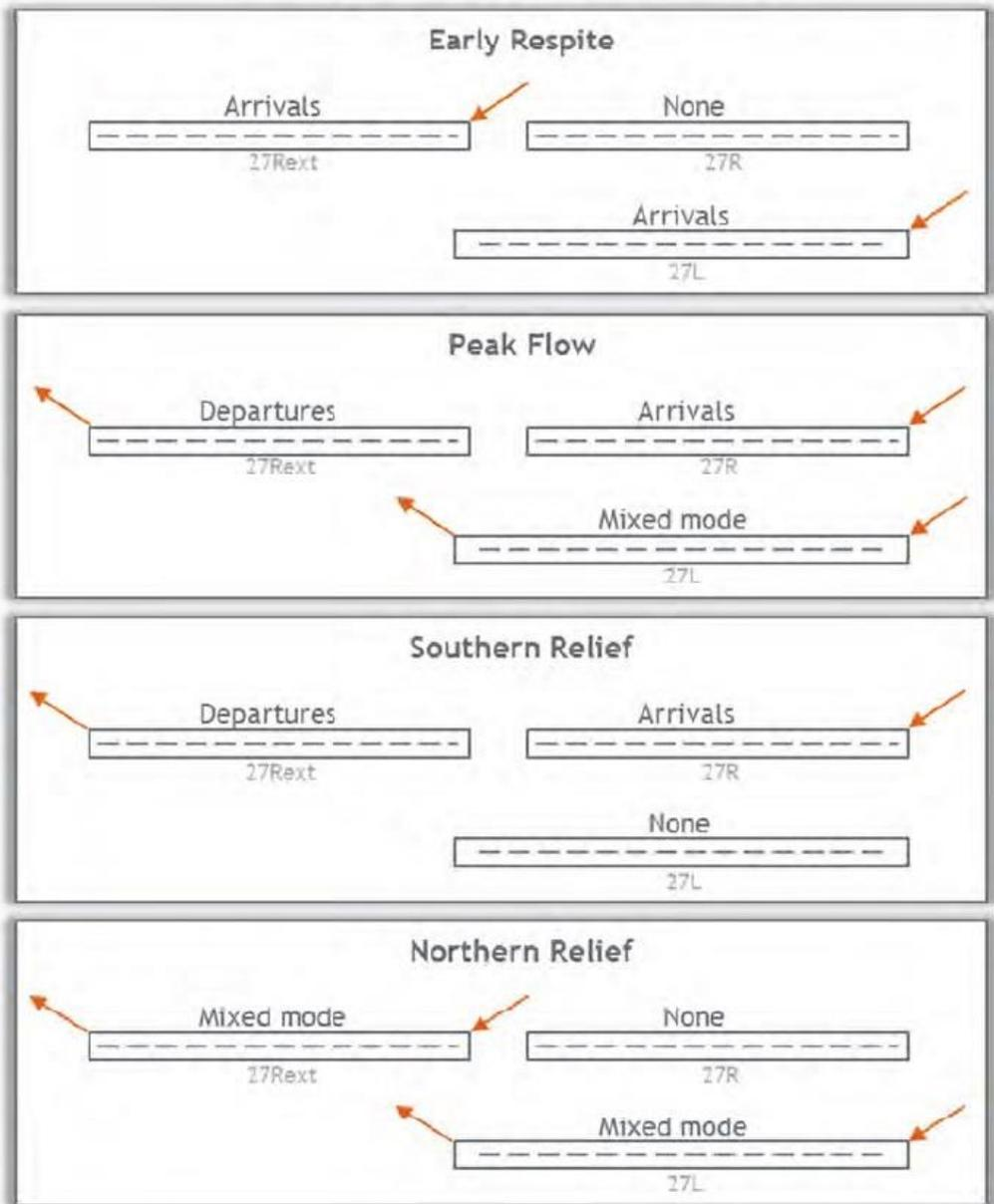
Figure 3-2 Heathrow Airport Extended Northern Runway Concept of Operating Modes (Source: Heathrow Hub Ltd submission to the Airports Commission)
