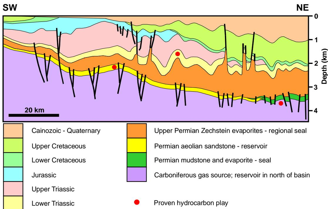
Fig. 12 Schematic section illustrating principal plays in the North Sea Gas Province. See Fig. 4 for location of section
