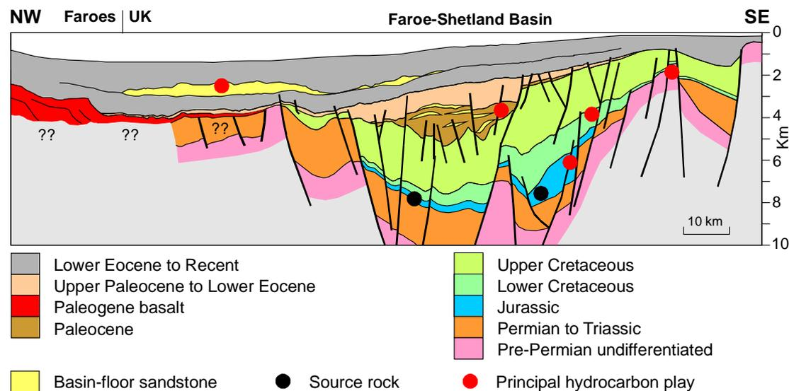
Fig. 22 Schematic play diagram for the Faroe-Shetland Basin. See Fig. 4 and 21 for location
