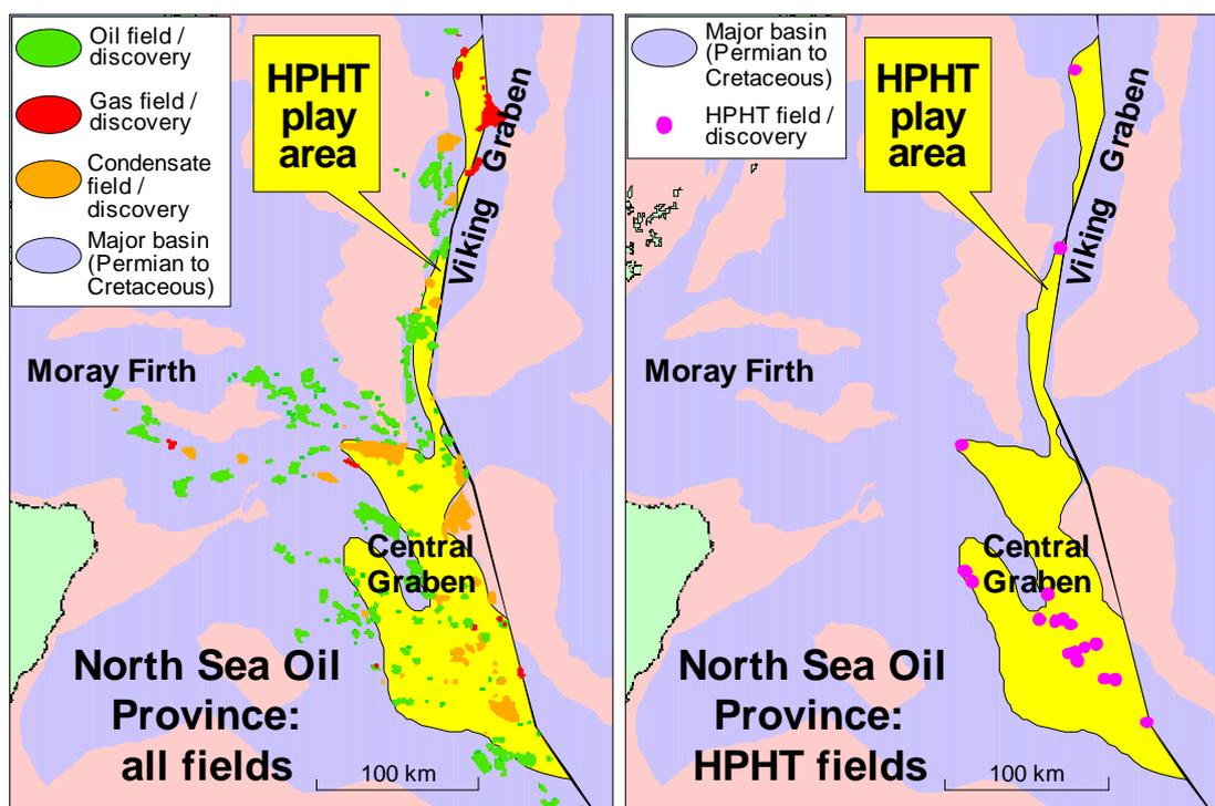
Fig. 7 Extent of the high pressure/high temperature (HPHT) gas condensate exploration play in the North Sea Oil Province
