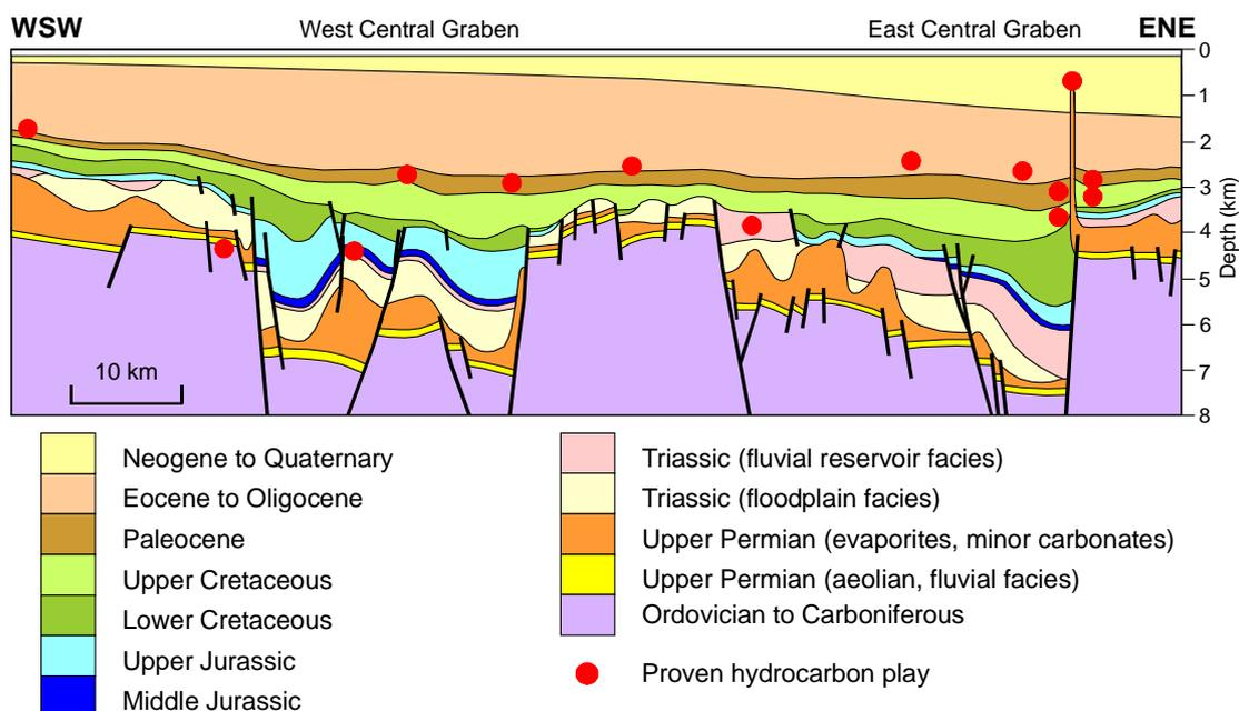
Fig. 10 Schematic section illustrating principal under-explored plays in the Central North Sea. See Fig. 4 for locations
