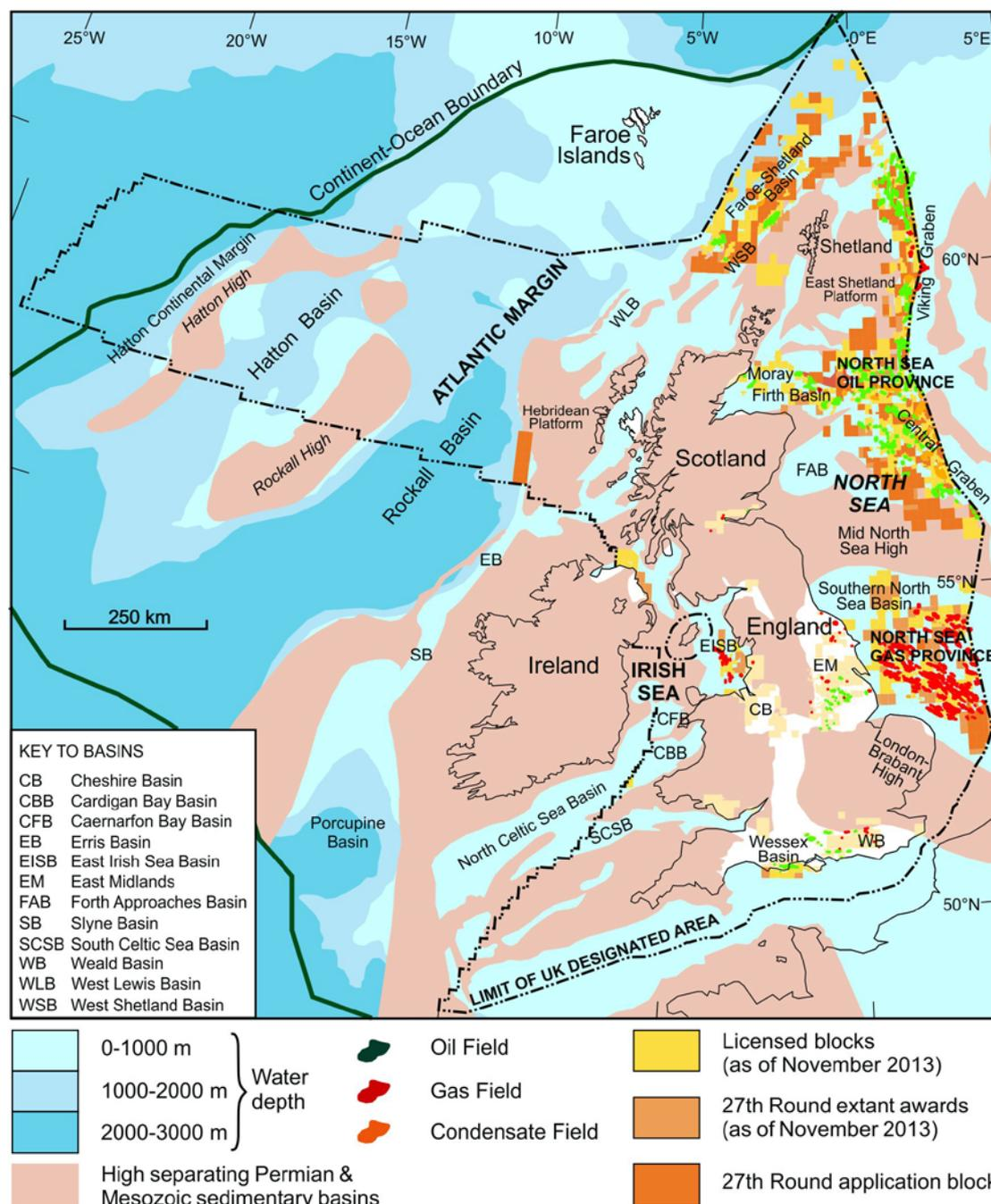
Fig. 1 Location of the hydrocarbon-producing basins and frontier basins of the UK and its designated waters
