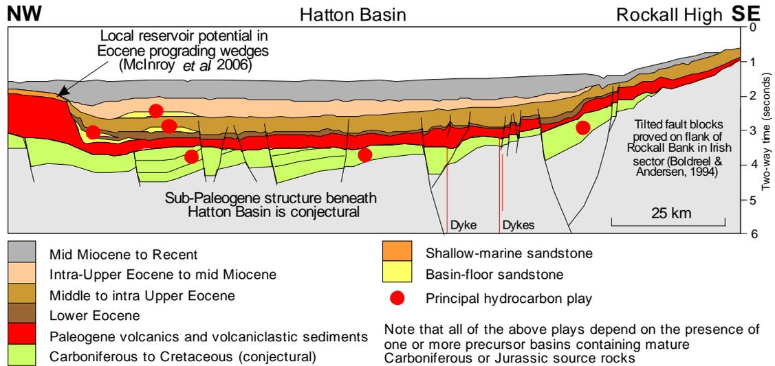
Fig. 25 Schematic play diagram for the Hatton Basin. See Fig. 20 for location
