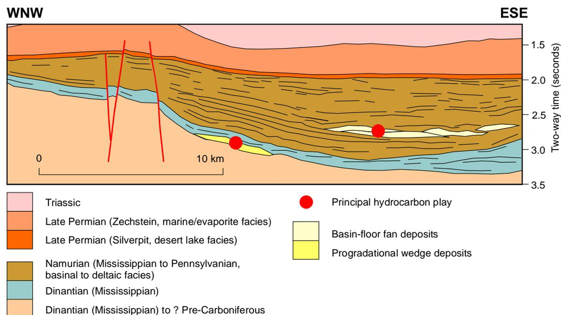
Fig 16 Geoseismic section illustrating undrilled Lower Carboniferous plays, North Sea Gas Province (adapted from Cameron and Ziegler 1997). See Fig. 14 for location
