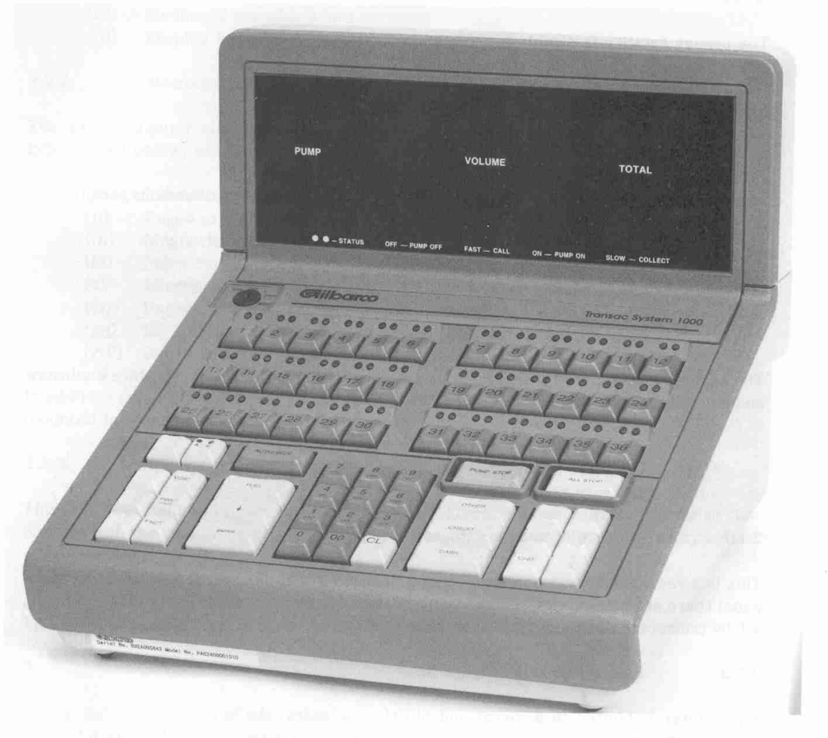
Figure 18 TS1000 kiosk control console (36 pump keys)
