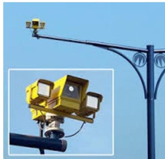
The set distance can be between two or more cameras, creating a speed control zone. In addition, the cameras are each fitted with infrared illuminators so they can operate at night or at times of poor daylight.
