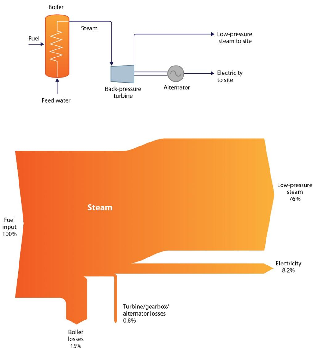
**Figure 12: Energy flow diagram for a steam turbine CHP**
