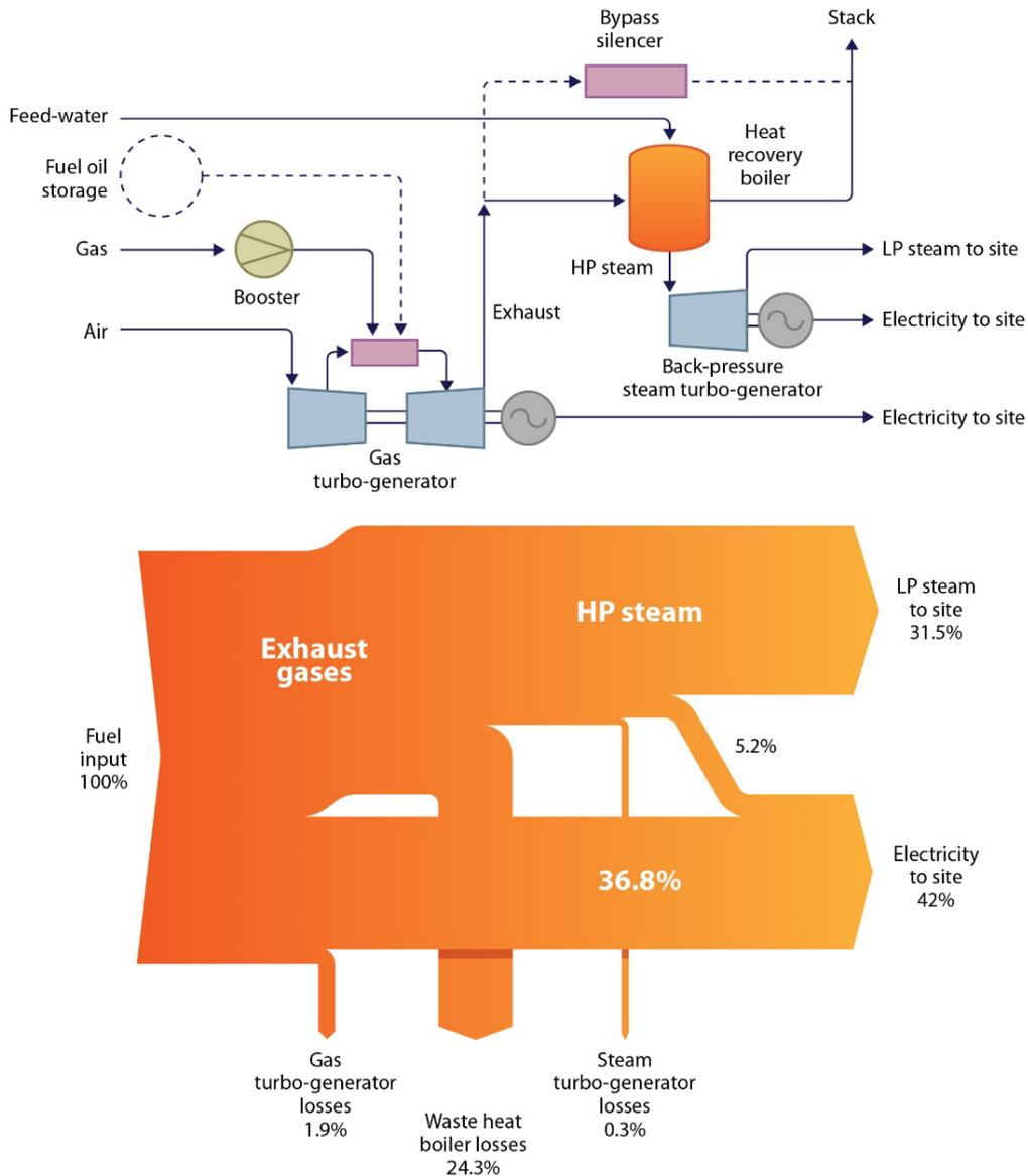
**Figure 13: Energy Flow diagram for a combined cycle gas turbine CHP**
