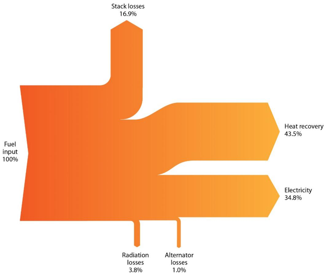
**Figure 9: Energy flow diagram for a CHP Engine with heat exchanger**
