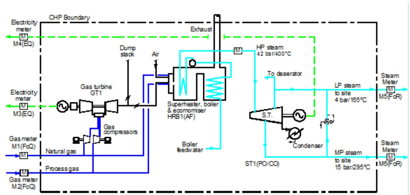
**Figure 1: A combined cycle gas turbine CHP**
