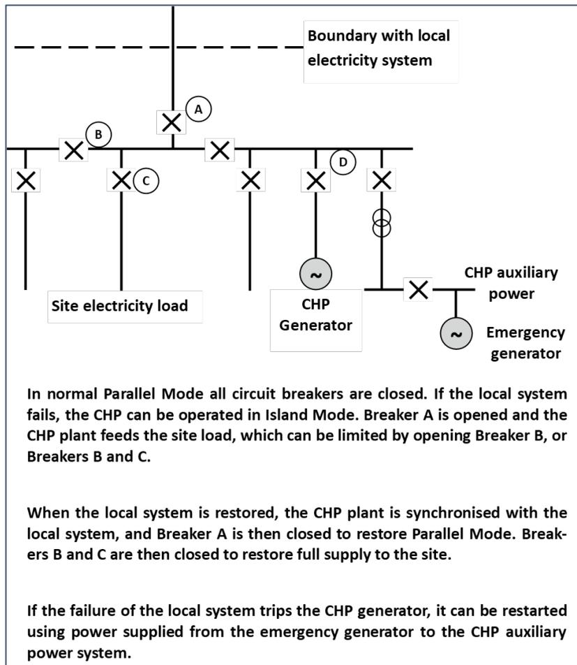
Figure 14 - Circuit Breaker Schematic
