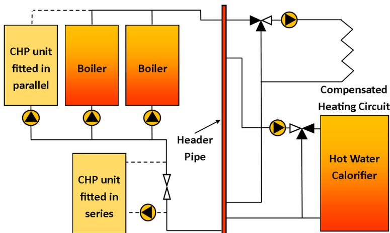
**Figure 5: A schematic diagram for a CHP Unit with boilers**
