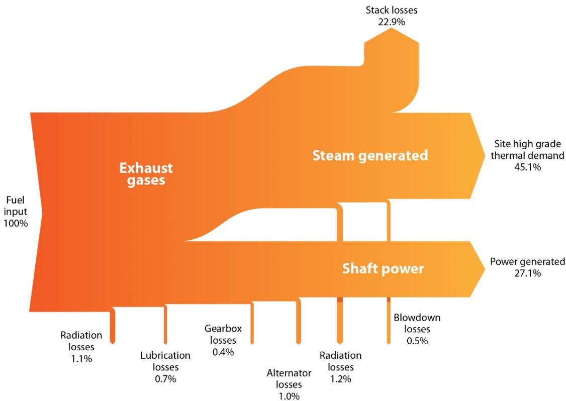
**Figure 7: Energy Flow Diagram for a gas turbine CHP**
