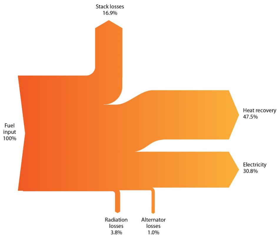
**Figure 3: Energy flow diagram for Reciprocating Engine CHP**
