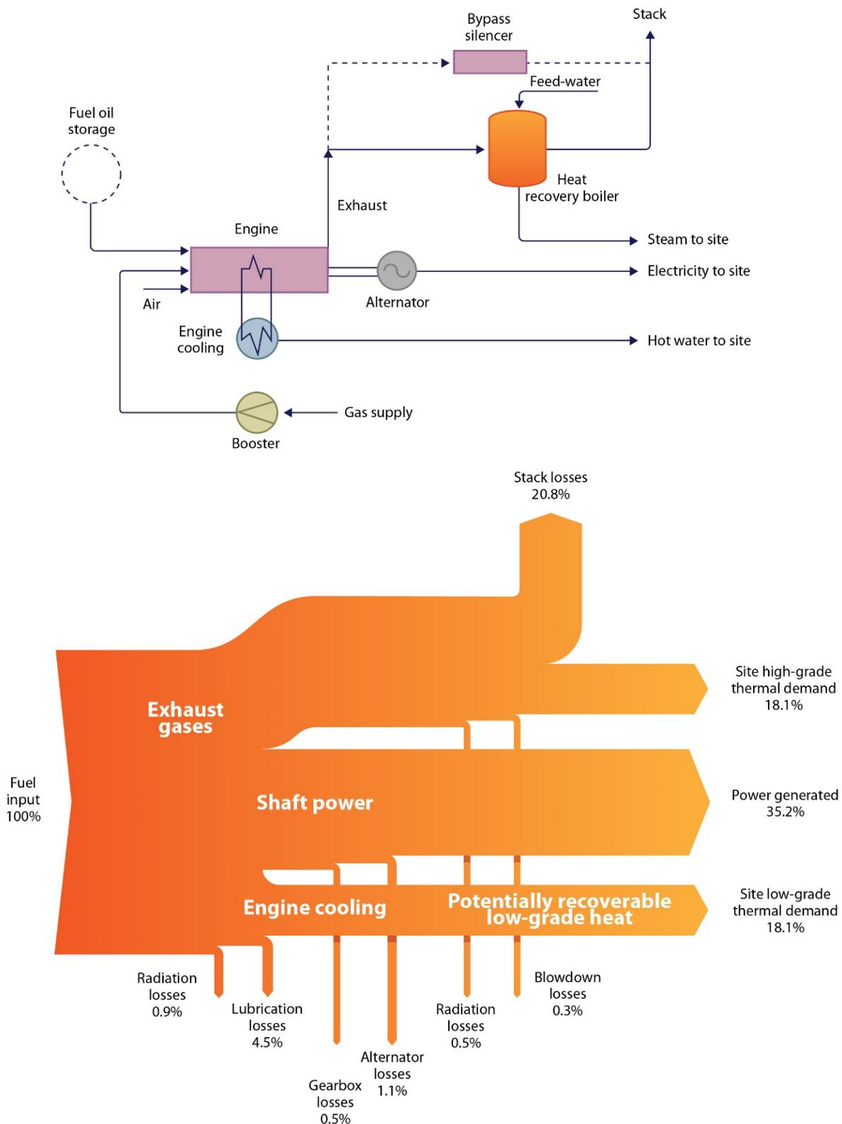
Figure 10: Energy flow diagram for a CHP engine with Heat Recovery Boiler
