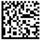
GS1 DataMatrix codes (see image, left) can be etched onto devices such as surgical instruments or printed on small packs, overcoming the size limitations of linear barcodes. RFID tags can be attached to a product, enabling its whereabouts to be located without line-of-sight scanning. GS1 DataMatrix and RFID tags can carry expiry date, batch number and serial number, supporting the EU unique device identification requirement.
