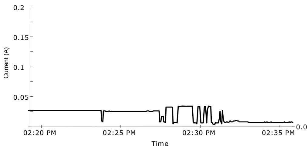
In a small number of situations isolated high P1 and or P2 spot measurements were attributed to the localised fields produced by point sources such as operating appliances in the home (Figure 9). Homeowners were asked whether any such appliance had been operating at the time of the original study measurements, and the original study EMF questionnaires were checked for any such evidence.
