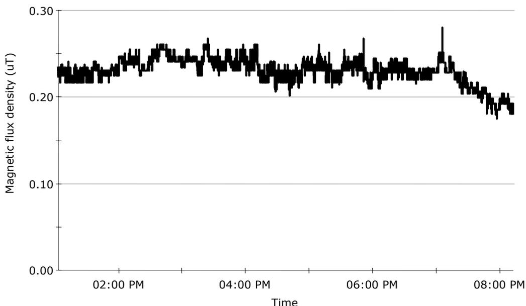
On the other hand, magnetic fields caused by net currents in distribution mains circuits tended to be more variable reflecting the complex relationship with the primary load currents. An example is shown in Figure 6.
