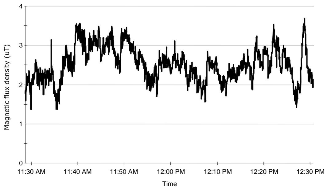
It was also possible to compare the traces from a field logger placed close to an external circuit with those from field loggers inside the home. Highly correlated traces such as those shown in Figure 6 provided evidence for the external circuit being the important source of the field inside the home.
