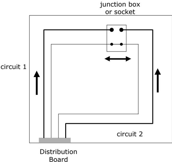
**Figure 17** Two-way lighting switch fault
