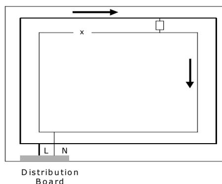
**Figure 16** Wiring fault caused by joining of neutrals in two radial circuits resulting in net currents in each circuit
