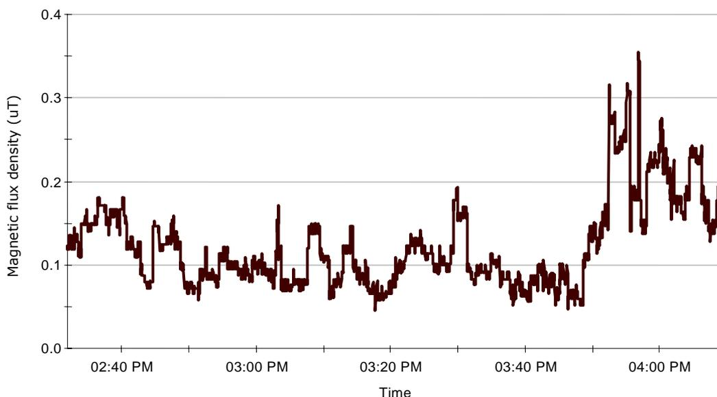
**Figure 22 Magnetic flux density recorded in a bedroom of a property with PME and with service neutral and conducting water piper shared with neighbouring properties. The magnetic field increased when a test load was applied in a neighbouring home**
