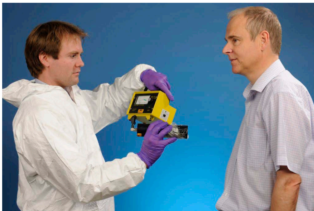
Figure C2 Monitoring of whole body activity with a hand-held radiation monitor
