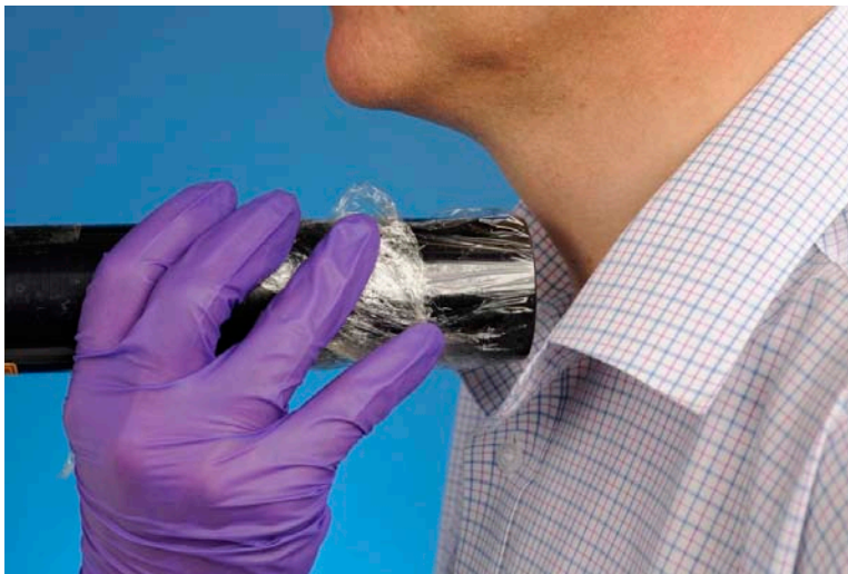
Figure C3 Monitoring of the thyroid for I-131 with a hand-held radiation monitor
