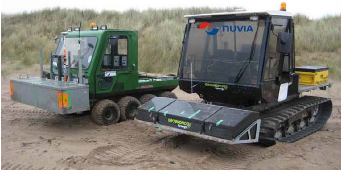
Figure 4: Vehicle mounted Groundhog beach detection systems (Evolution 2™ on left; Synergy on right) (copyright Sellafield Ltd)
