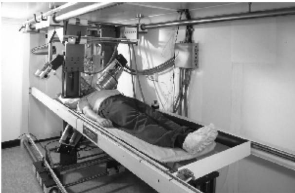
**Figure 3: Low Background In vivo Detector Array (LBIDA) using Sodium Iodide detectors to measure head activity**
