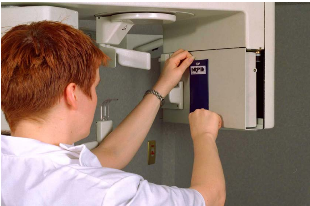
Figure 2 Showing use of panoramic test pack
