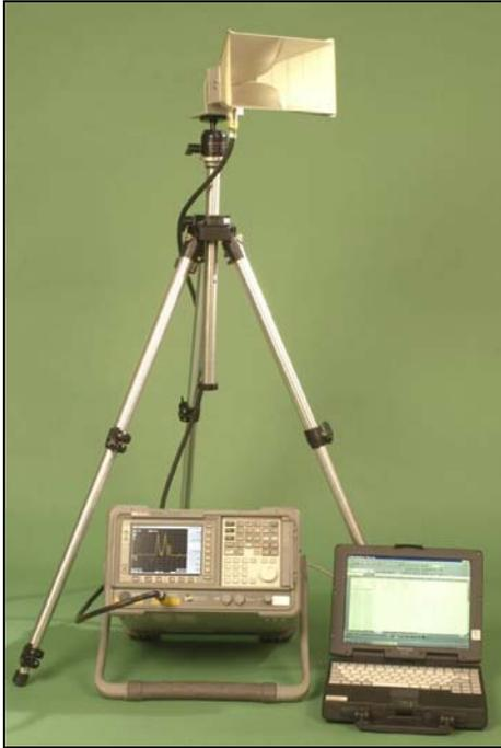
**FIGURE 3** Narrowband measurement equipment consisting of a spectrum analyser connected to a ridged guide horn antenna mounted on a tripod. A computer is used to capture, and subsequently process, the data
