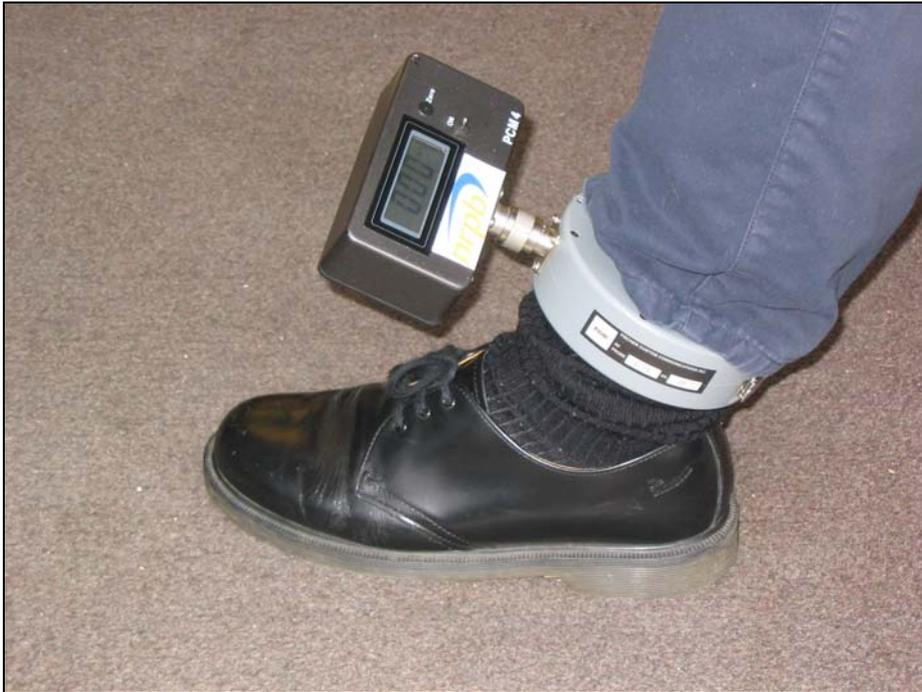
**FIGURE 5** Limb current meter consisting of a current transformer, clamped around the ankle, connected to a PCM4
