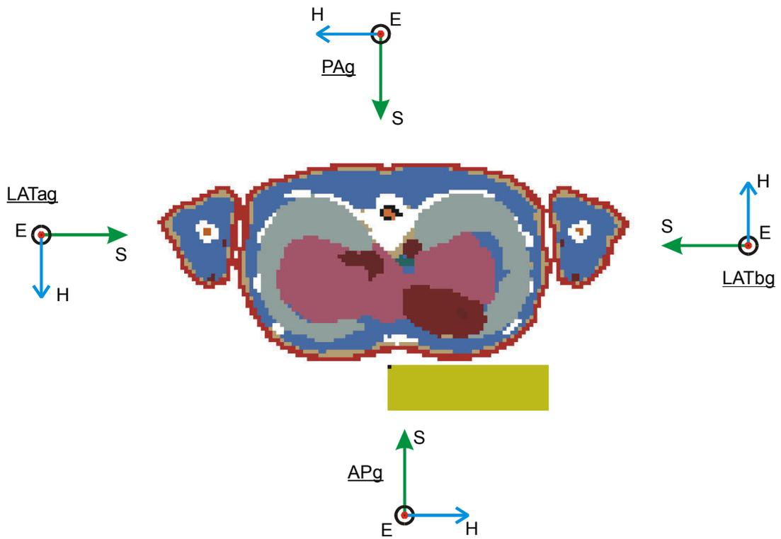
**FIGURE 9** Cross-sectional view of NORMAN from above showing the volume in which the field distribution was examined and the four plane-wave exposure conditions
