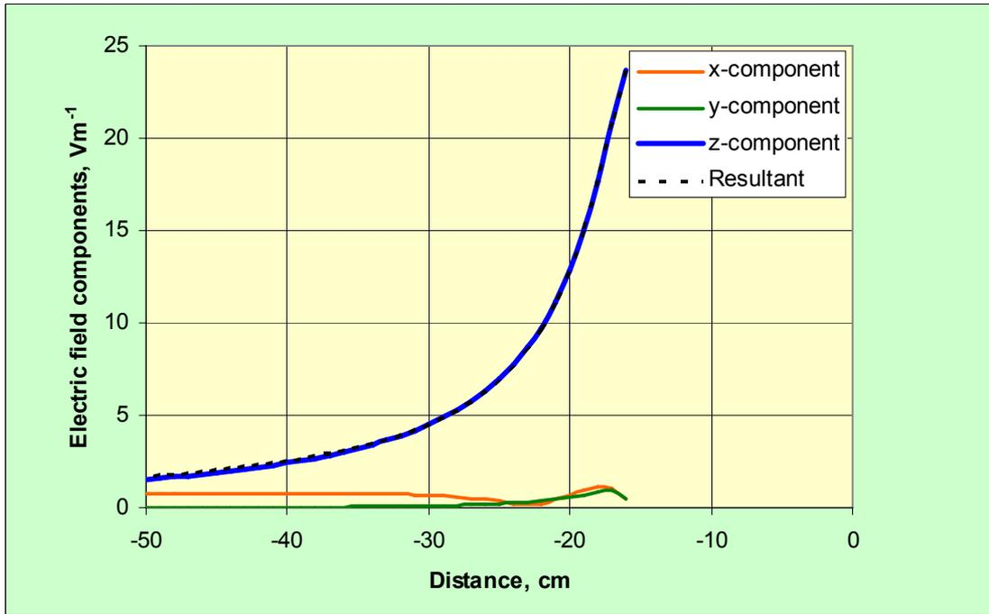
Figure A6 The components of electric field strength and the resultant as a function of distance along the negative z-direction at x = -2 cm and y = 0 cm
