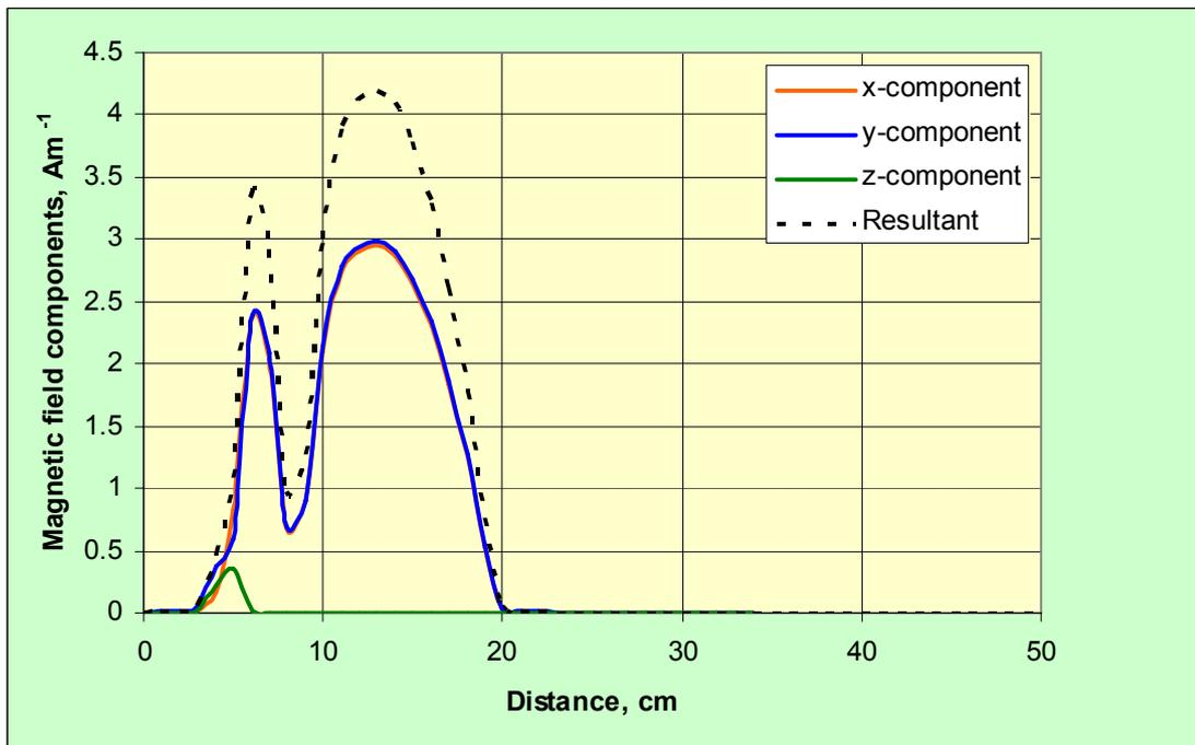
Figure A15 The components of magnetic field strength and the resultant as a function of distance along the positive z-direction at  $x = 3$  cm and  $y = 0$  cm
