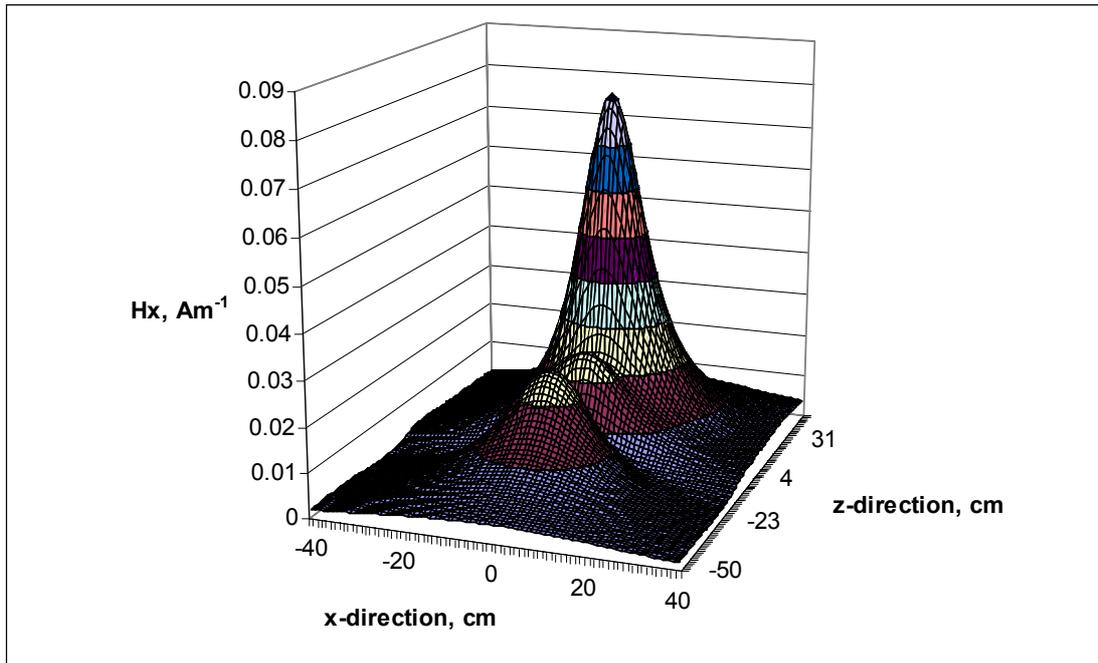
Figure A17 The x-component of magnetic field as a function of x and z at a displacement of 7 cm from the transponder along the negative y-direction
