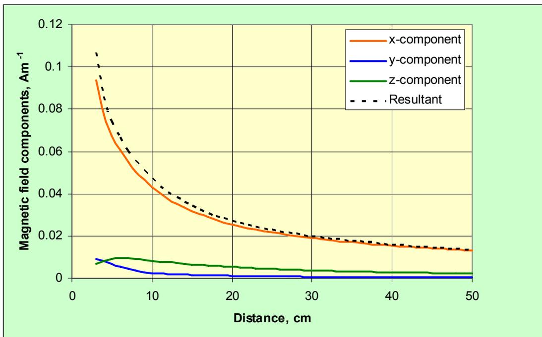
Figure A12 The components of magnetic field strength and the resultant as a function of distance along the positive y-direction at  $x = 3$  cm and  $z = 9$  cm
