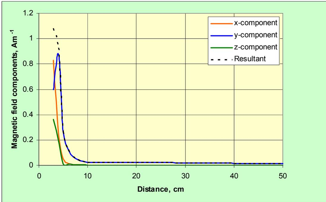
Figure A14 The components of magnetic field strength and the resultant as a function of distance along the positive x-direction at  $y = 0$  cm and  $z = 9$  cm
