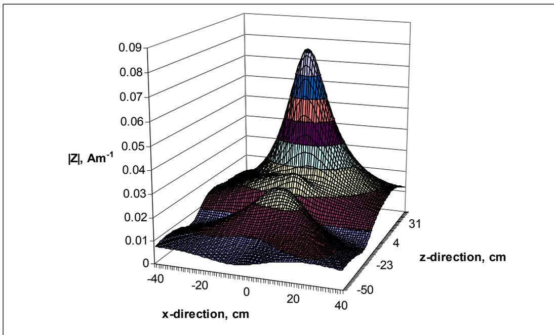
Figure A20 The resultant magnetic field as a function of x and z at a displacement of 7 cm from the transponder along the negative y-direction
