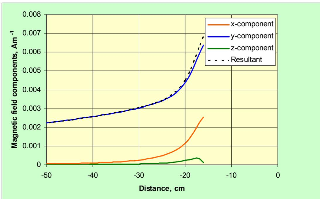
Figure A16 The components of magnetic field strength and the resultant as a function of distance along the negative z-direction at  $x = -2$  cm and  $y = 0$  cm
