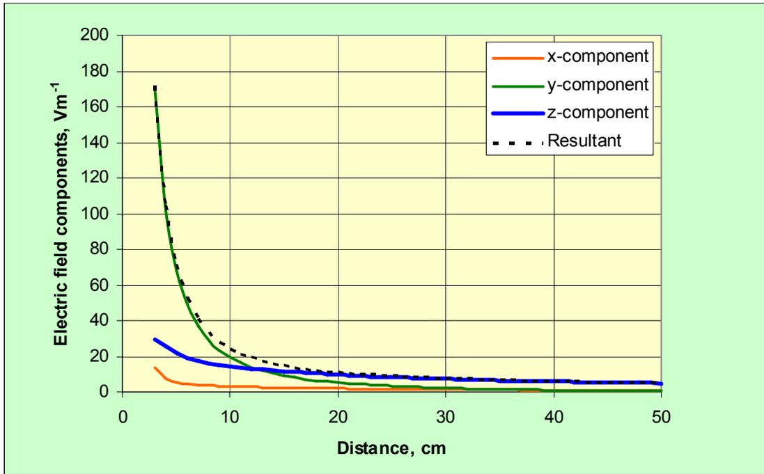
Figure A2 The components of electric field strength and the resultant as a function of distance along the positive y-direction at x = 3 cm- and z = 9cm
