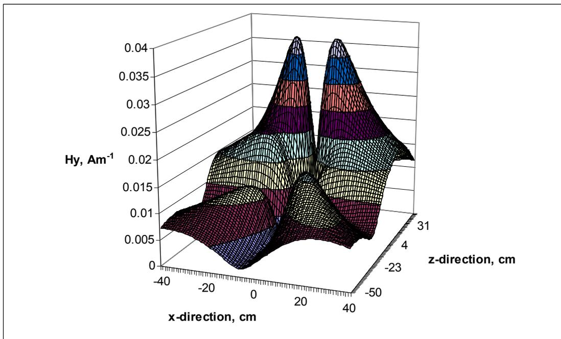
Figure A18 The y-component of magnetic field as a function of x and z at a displacement of 7 cm from the transponder along the negative y-direction
