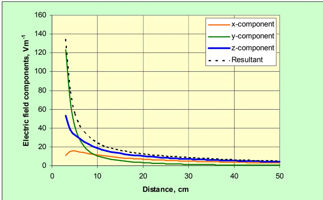
Figure A21 The components of electric field strength and the resultant as a function of distance along the negative y-direction at x = 3 cm and z = 9 cm
