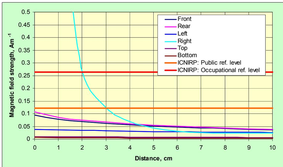
Figure 7 Magnetic field strength as a function of distance from various sides of the transponder in relation to the ICNIRP reference levels
