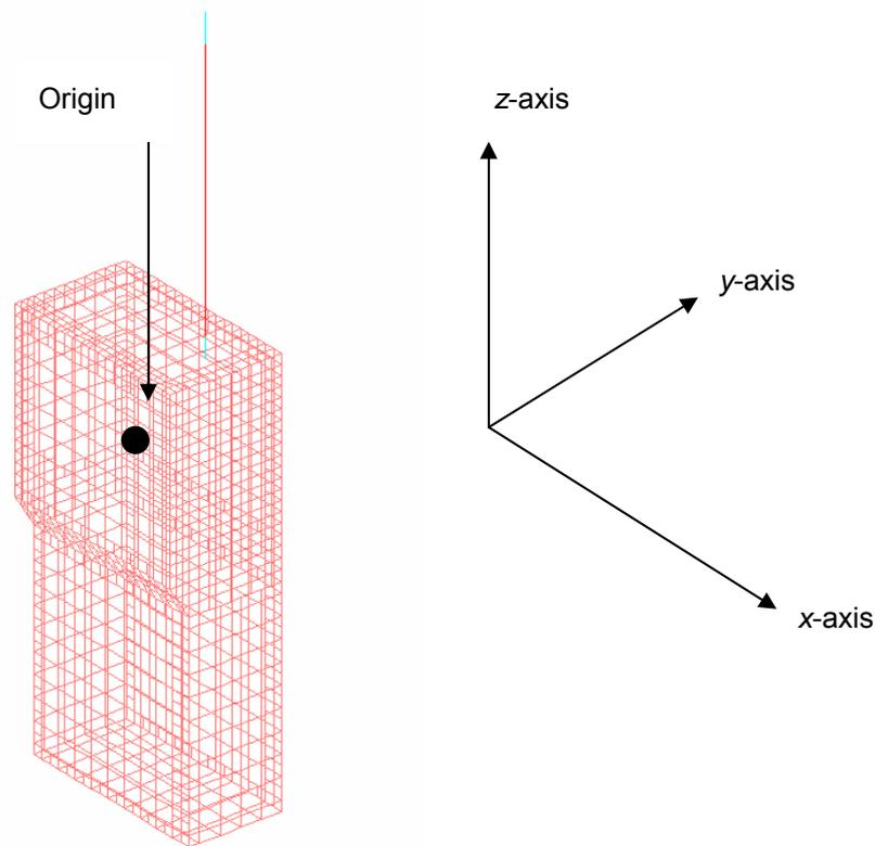
**Figure 5 NEC model of the Mode S transponder with a monopole antenna**
