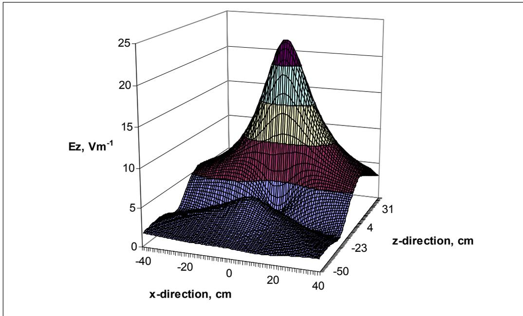
**Figure A9** The z-component of electric field as a function of x and z at a displacement of 7 cm from the transponder along the negative y-direction
