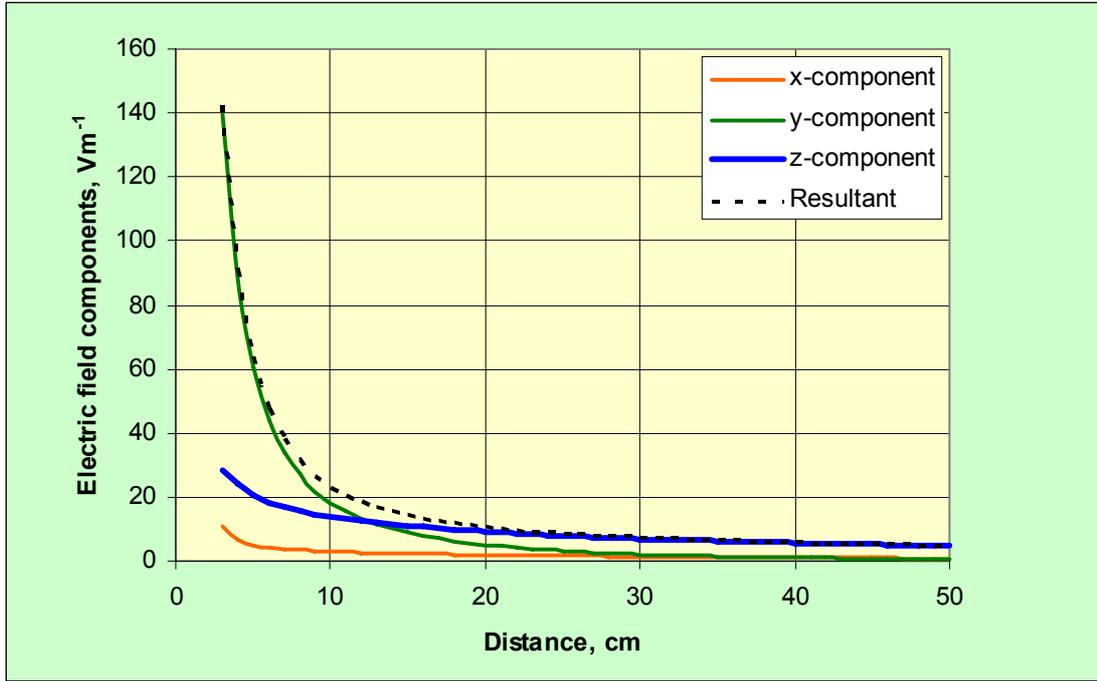
Figure A1 The components of electric field strength and the resultant as a function of distance along the negative y-direction at x = 3 cm- and z = 9cm
