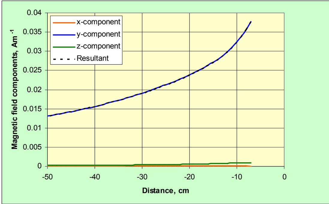
Figure A13 The components of magnetic field strength and the resultant as a function of distance along the negative x-direction at  $y = 0$  cm and  $z = 5$  cm
