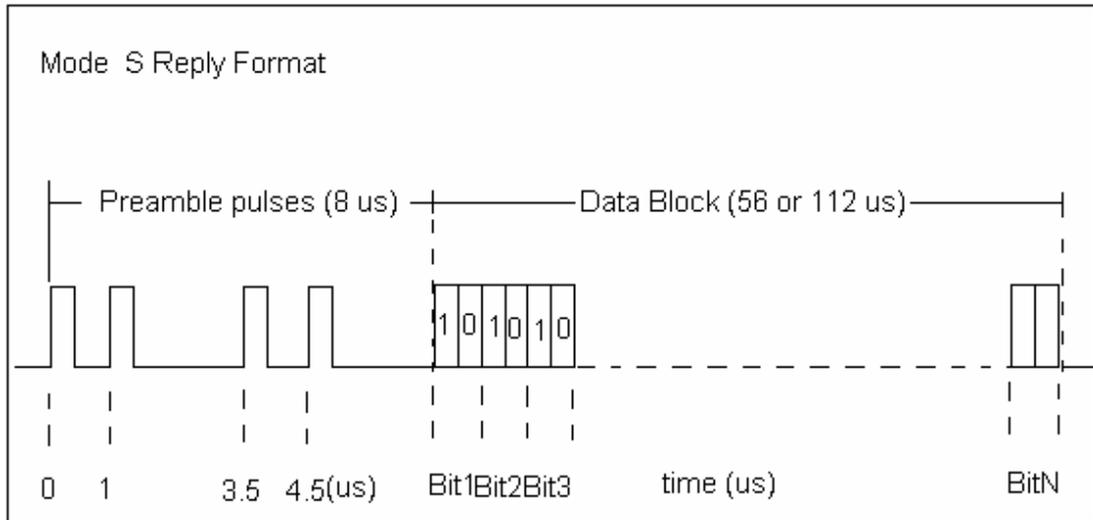
**Figure 3 Mode S reply format**
