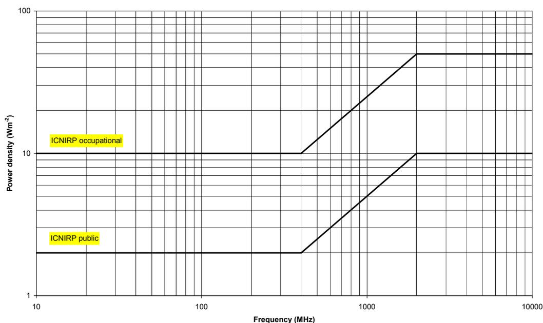
Figure 4 ICNIRP reference levels for power density at frequencies between 10 MHz and 10 GHz
