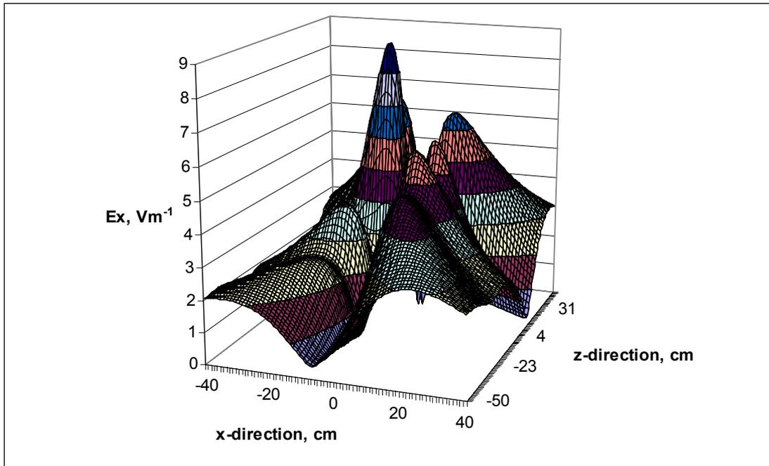
Figure A7 The x-component of electric field as a function of x and z at a displacement of 7 cm from the transponder along the negative y-direction
