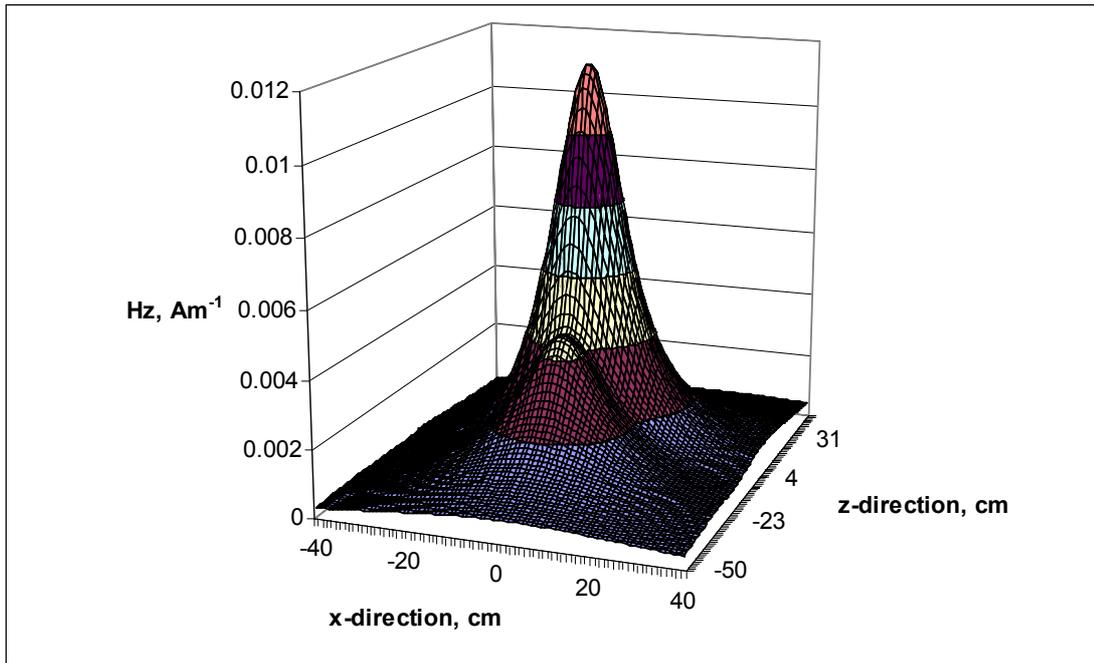
Figure A19 The z-component of magnetic field as a function of x and z at a displacement of 7 cm from the transponder along the negative y-direction
