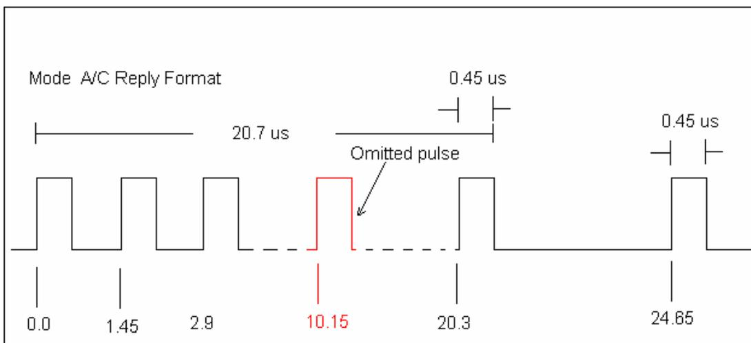
Figure 2 Mode A/C reply format
