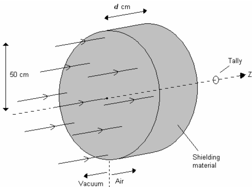
Figure 1: Geometry of the modelled configuration, with the source impinging from the left.
