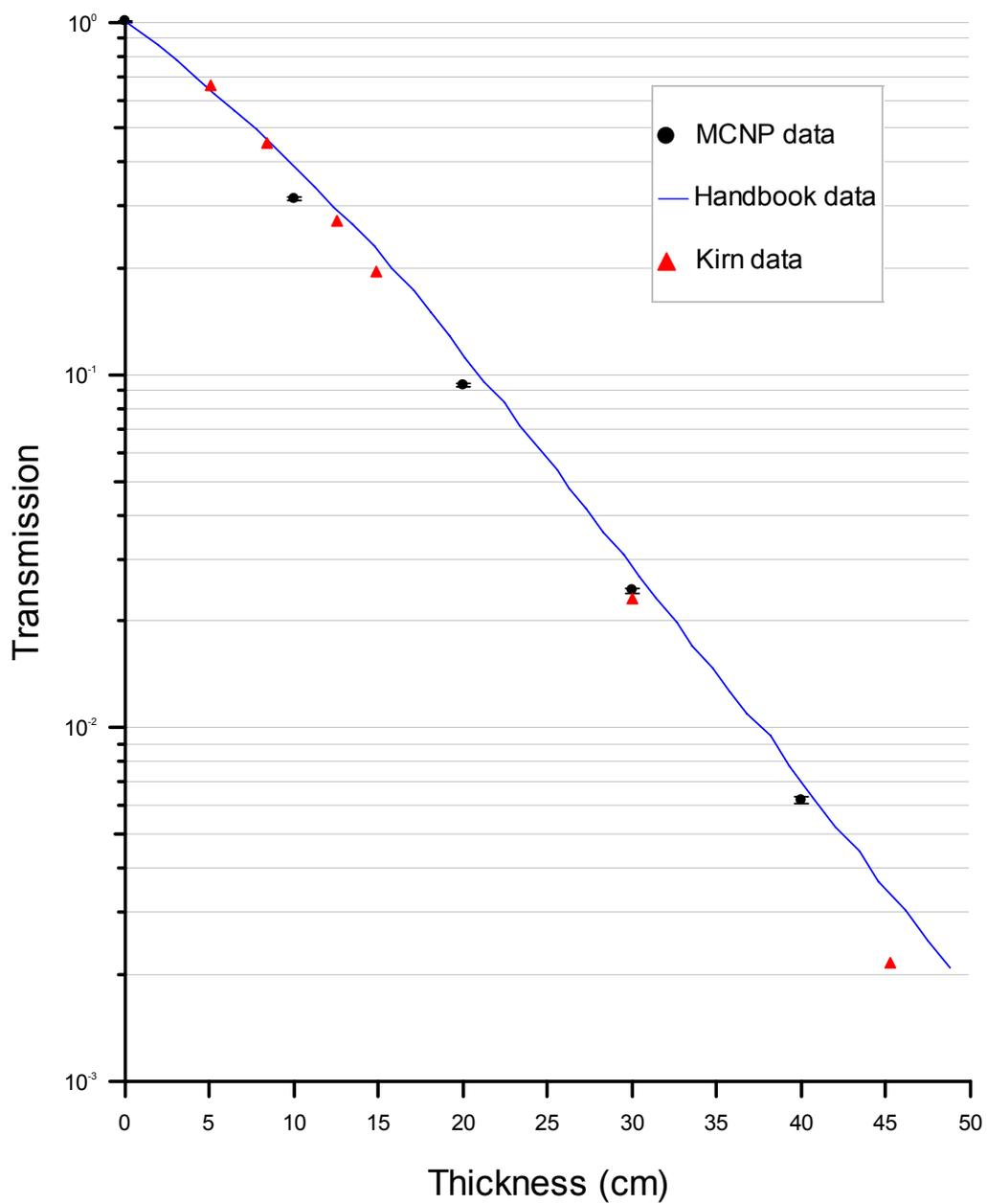
Figure 2: Transmission of 0.662 MeV gamma rays through concrete. Both MCNP and experimental results are presented.
