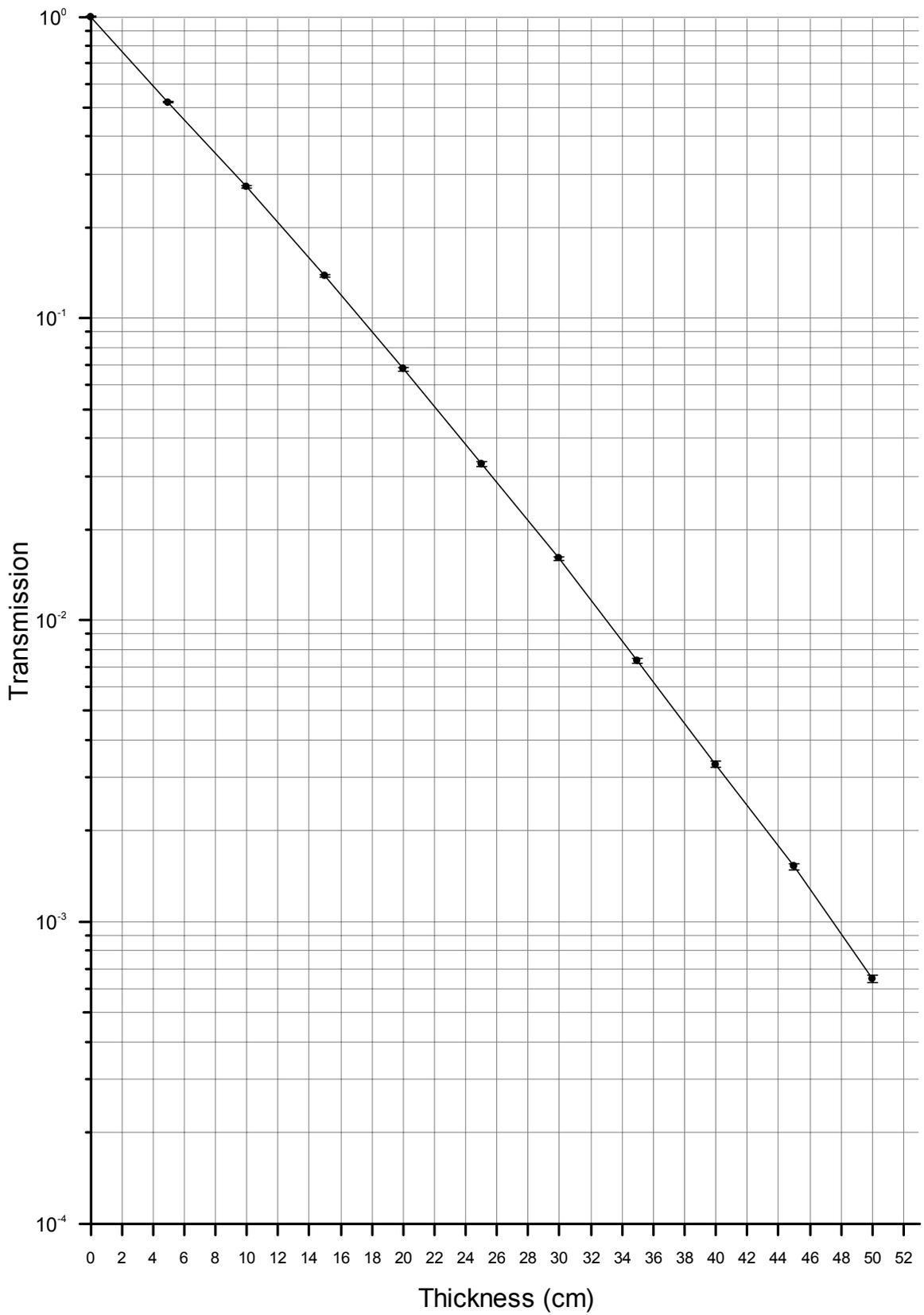
Figure 3: Transmission of 0.511 MeV gamma rays through concrete.
