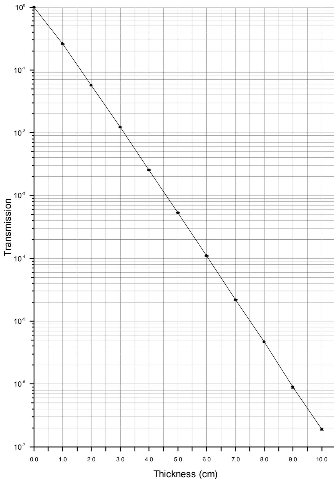
Figure 4: Transmission of 0.511 MeV gamma rays through lead.
