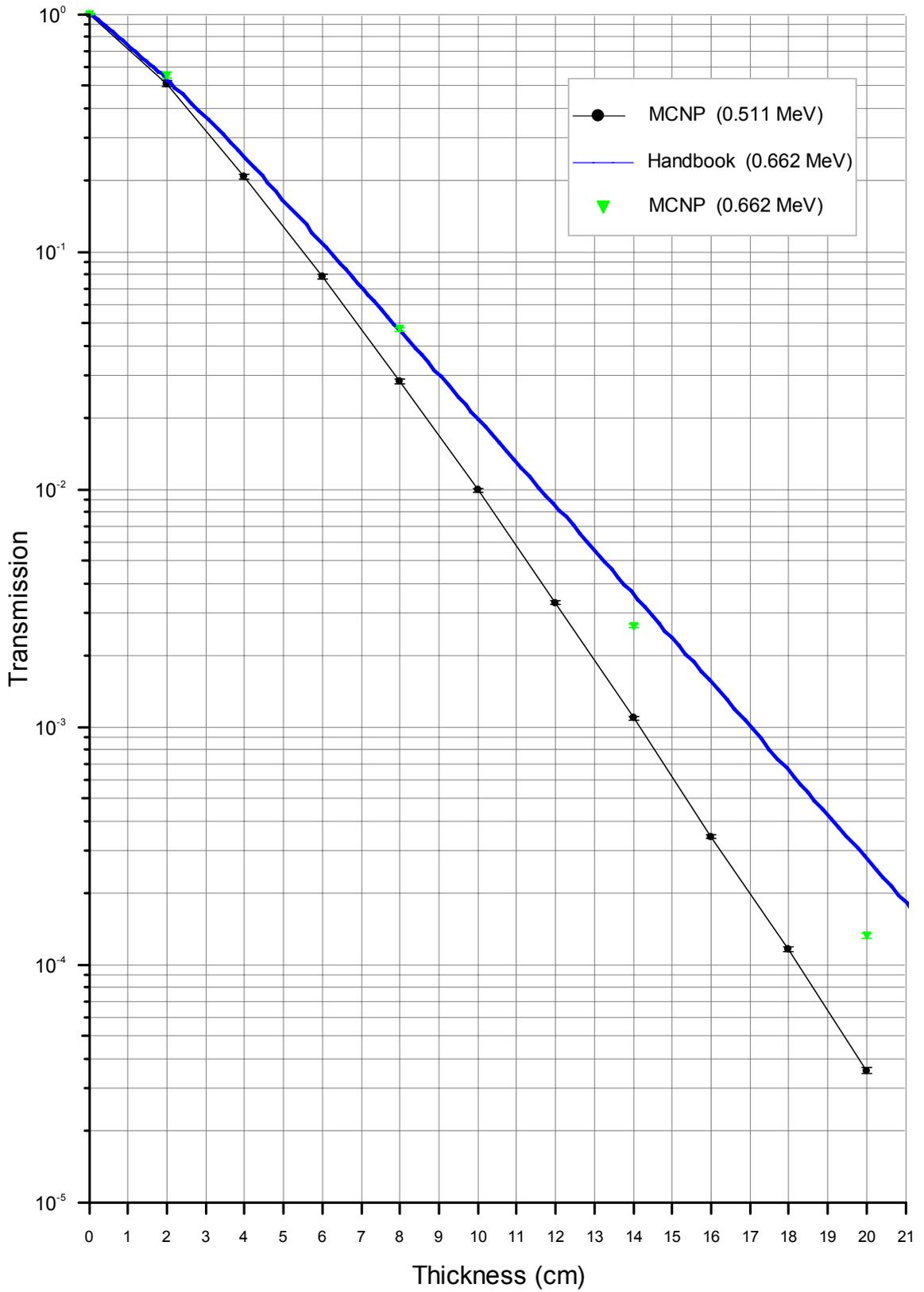
Figure 5: Transmission of 0.511 MeV gamma rays through iron. Also presented are the HRP and MCNP data for the Cs-137 gamma ray transmission through iron.
