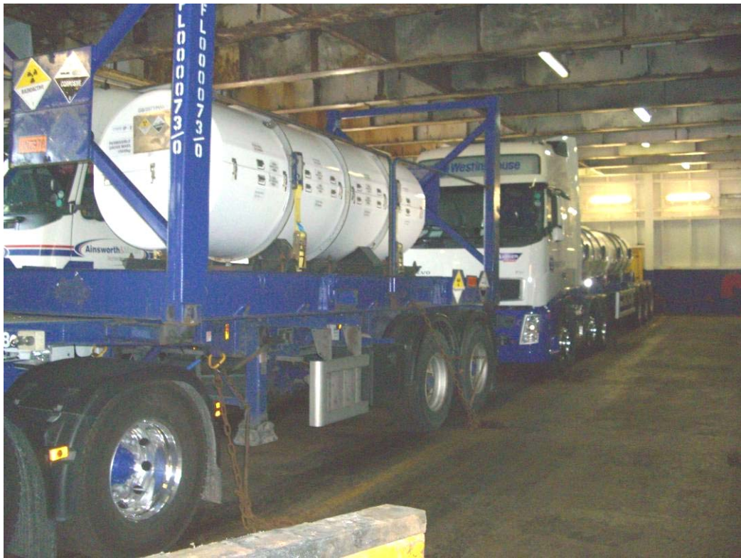
Figure 3. Lorries carrying 48Y cylinders of natural UF 6 on the vehicle deck of a freight ferry
