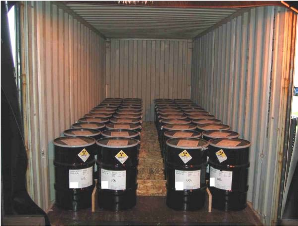
Figure 2. Drums of UO 3 inside a freight container
