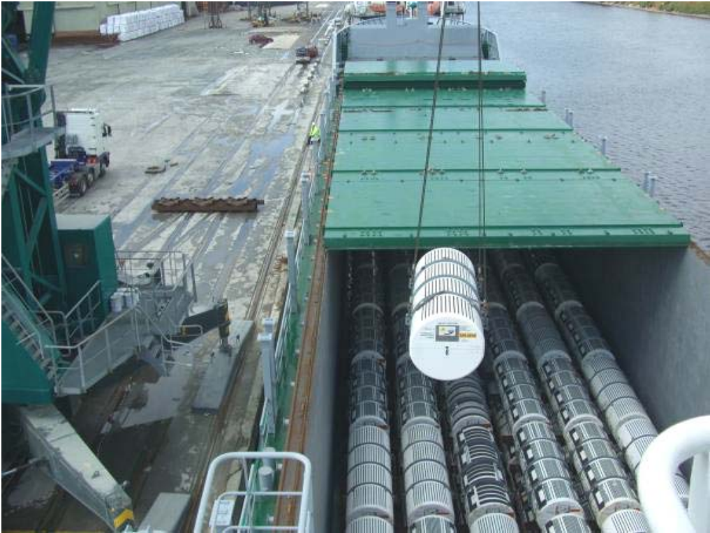
Figure 8. Loading of cylinders of depleted UF 6 into the hold of a ship
