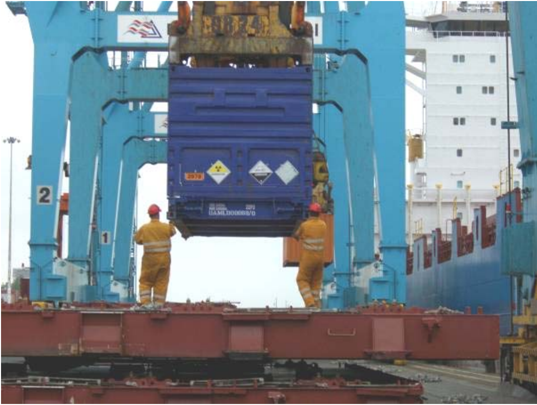
Figure 4. Manual removal of twist locks
