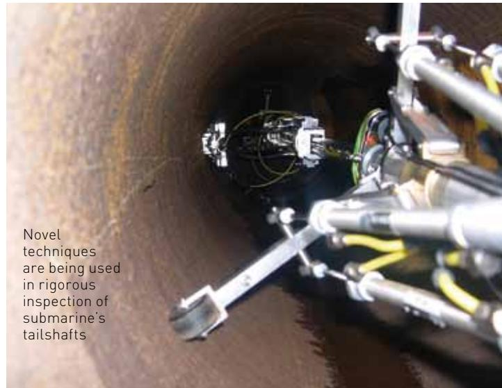
Novel techniques are being used in rigorous inspection of submarine's tailshafts
