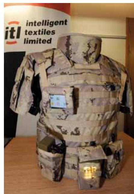
Above: Intelligent Textiles' new conductive body armour material with some ancillary items connected via USB ports
