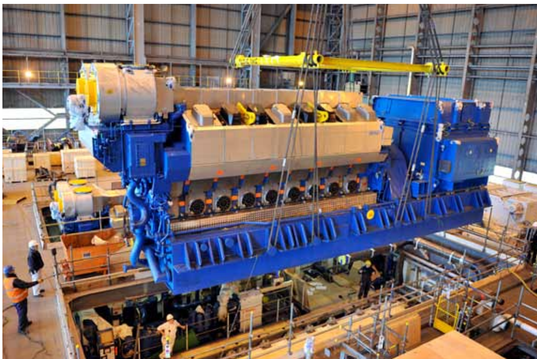
A diesel generator is lowered into place at BAE Systems' yard at Govan
