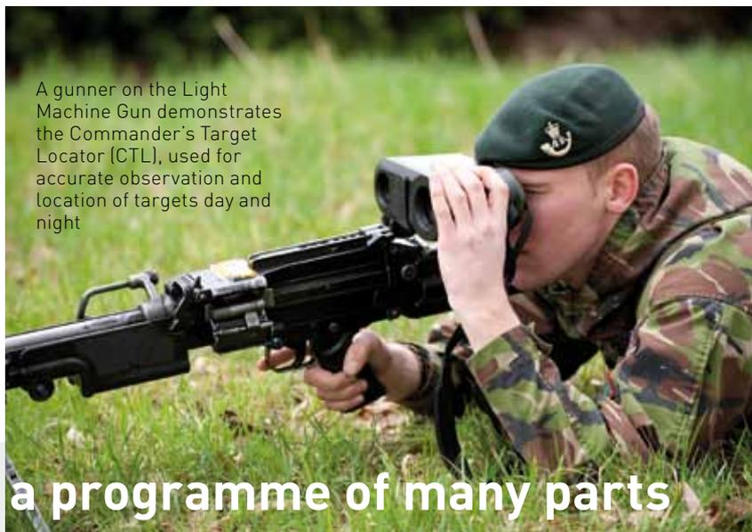
A gunner on the Light Machine Gun demonstrates the Commander's Target Locator (CTL), used for accurate observation and location of targets day and night
