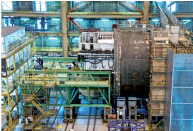
Left: the manoeuvring room module is moved into Boat 3 Audacious at Barrow
