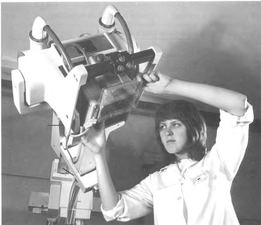
**FIGURE 4** Ionisation chamber of a dose–area product meter being attached to the diaphragm housing
