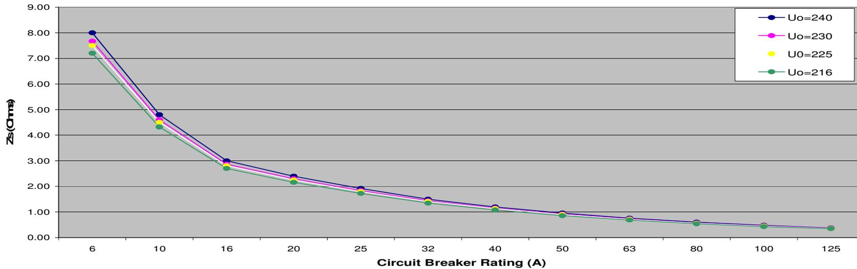
Figure D1: Values of Maximum Z<sub>s</sub> for Type B Circuit Breakers for 0.4 s disconnection time at various values of U<sub>o</sub>.
