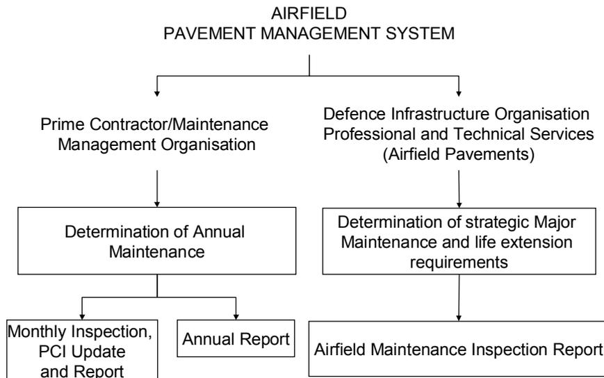
**Figure 1. Elements and responsibilities within the Pavement Management System**
