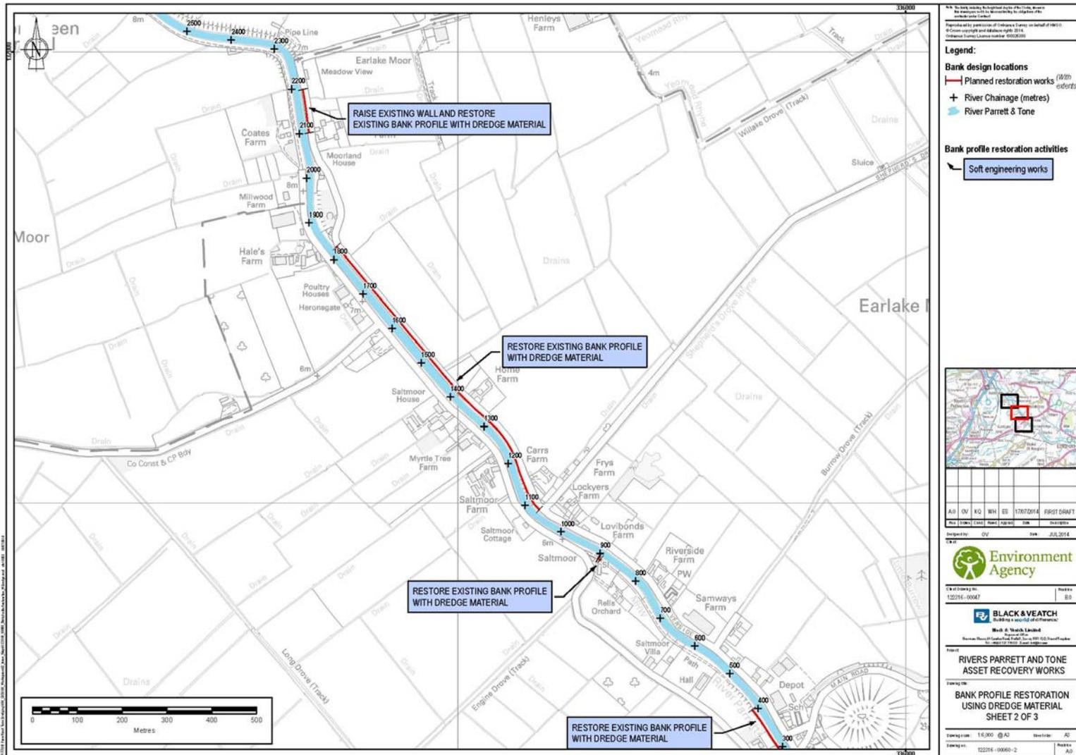
Figure 3b: Proposed Locations of Bank Profile Restoration
