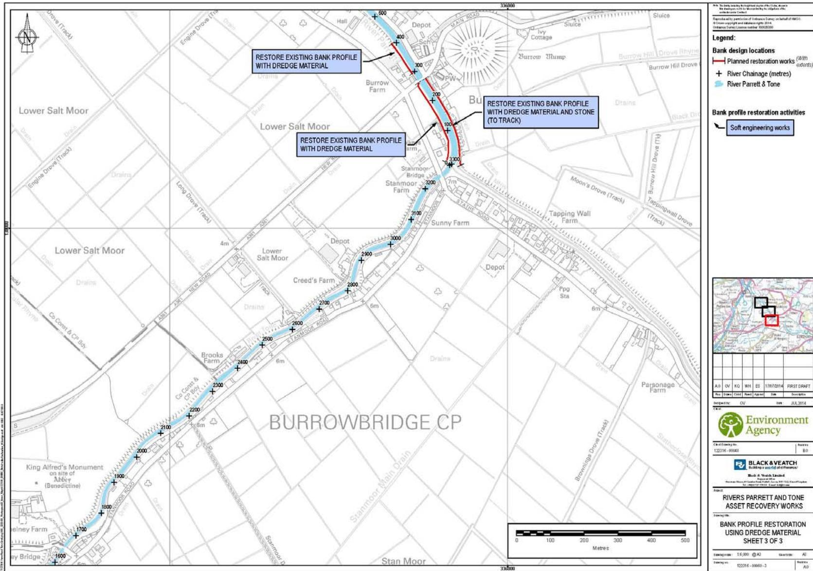
**Figure 3c: Proposed Locations of Bank Profile Restoration**
