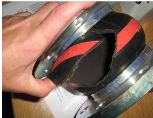
Figure 1 - Single red band - LTHW rated expansion bellows
