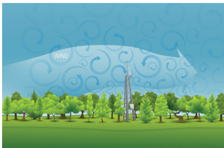
Figure 5.1 Eddy covariance schematic showing turbulent eddies in the Earth's boundary layer and a typical eddy covariance flux tower
