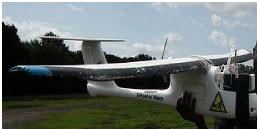
Figure 4.4 Integrated ozonesonde and Skywalker airframe
