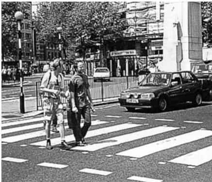
Where a crossing is thought necessary but crossing flows are relatively low and traffic flows are no more than moderate, then a Zebra crossing may be suitable. Pedestrians establish precedence by stepping onto the crossing and so delays to them are minimal. Vehicle delays are typically five seconds for a single able person crossing but can be much more where irregular streams of people cross over extended periods.
