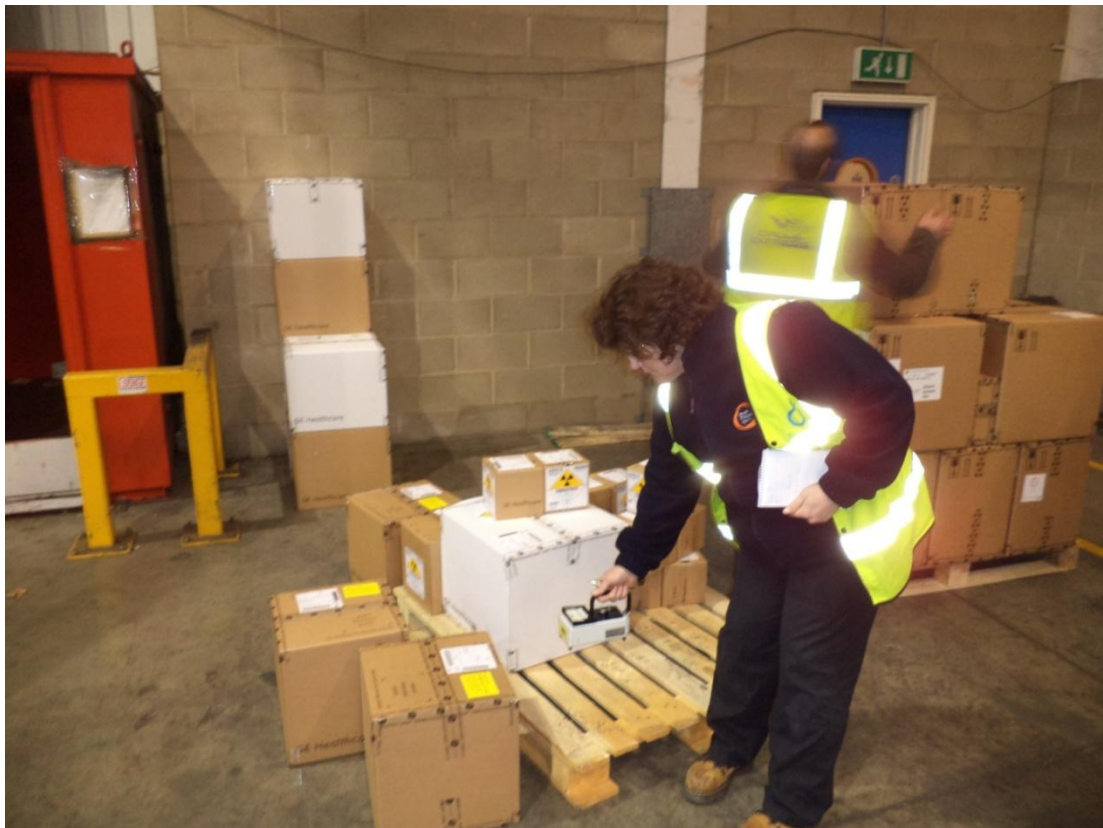
FIGURE 6 Measuring dose rates of packages before they are stored in the radiation store
