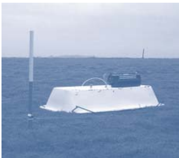
Figure 2.1 A typical flux box and methane detector set up for field measurements
