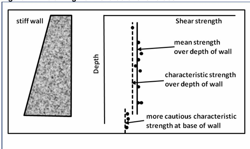
The active pressures on the back of the wall are derived from the characteristic value derived from the mean strength of the ground over the full depth of the wall.
