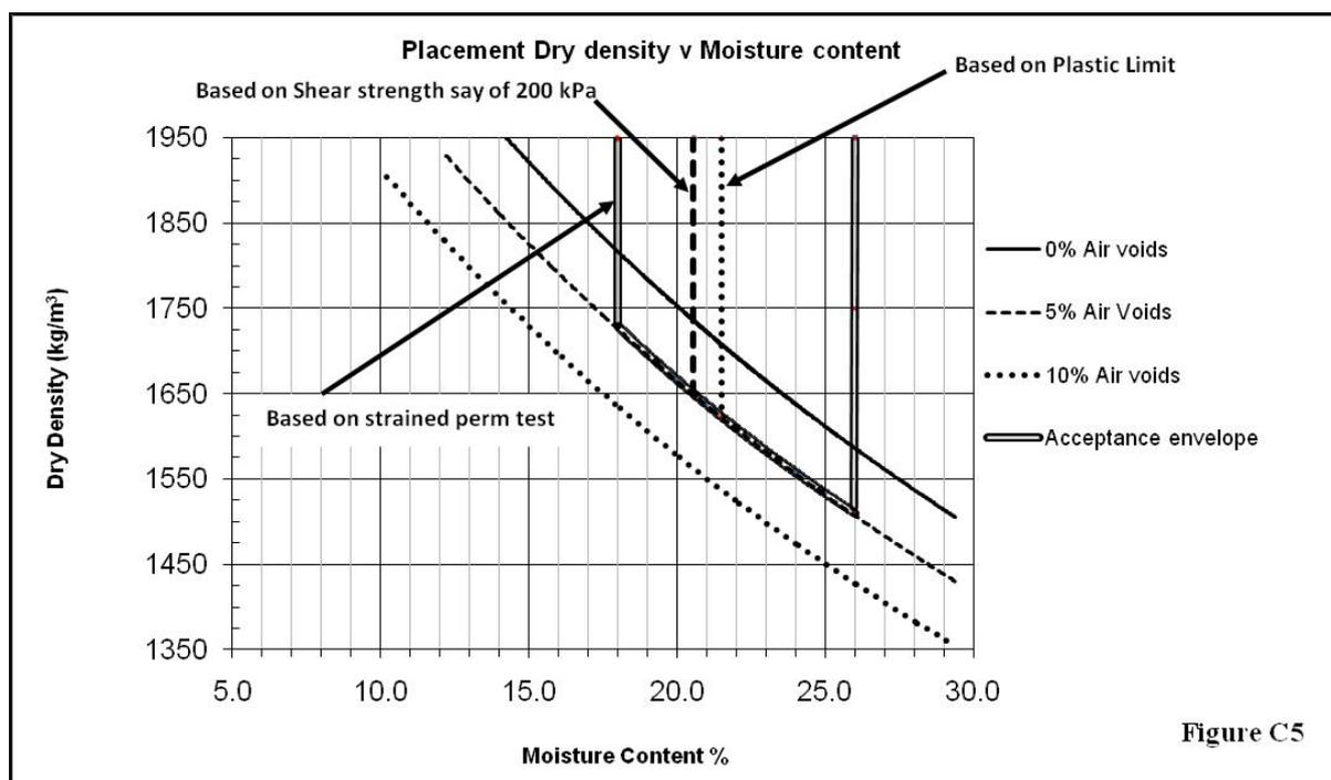
Control on site is by measuring dry density and moisture content, using a nuclear density meter, core cutter or by sand or water replacement, plotting the result on the graph and appraising pass or fail with this zone (see Appendix D).
