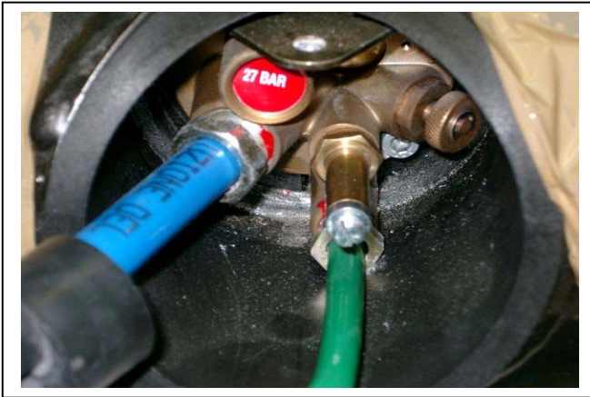
Electric Valve with Supplementary Manual Screw:
