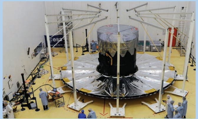
Gaia's heat shield being tested, the ESA spacecraft is due for launch in December 2013 Credit: ESA
