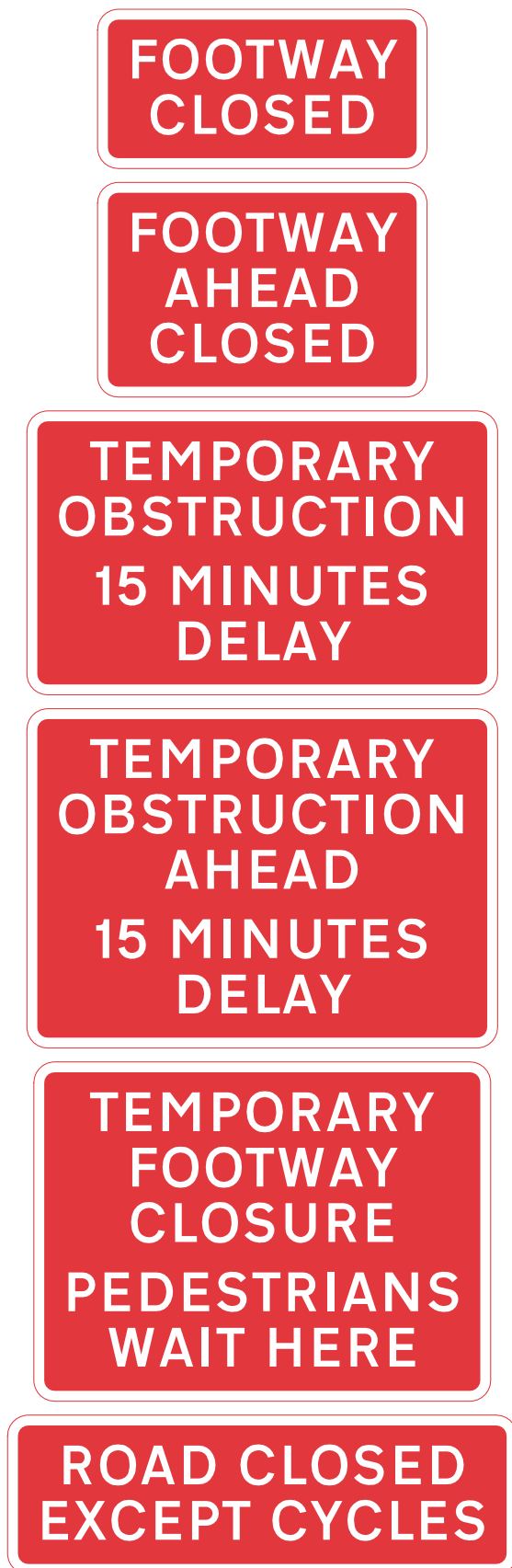
Figure 2 Some examples of signs allowed under regulation 53.
