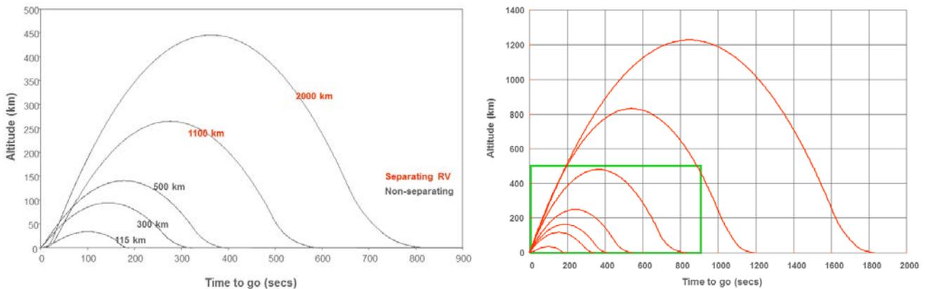
Figure 2: Trajectories associated with Short and Medium Range (left) and Intermediate Range and Intercontinental (right) Ballistic Missiles. The over-ground range of the system is shown next to each line on the left, and the green box on the right contains each of the trajectories detailed on the left.
