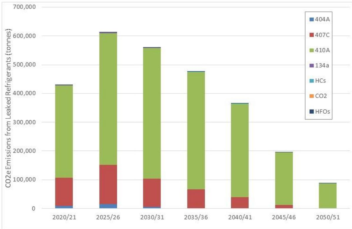
**Figure 25: CO<sub>2</sub>e Emissions due to Refrigerant Leakage to 2050/51 (tonnes) (including AAHPs)**
