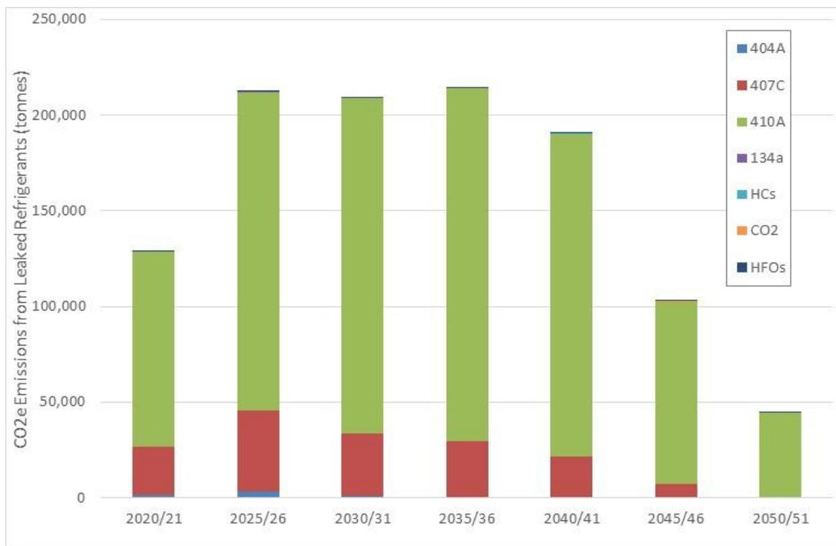
Figure 24: CO<sub>2</sub>e Emissions due to Refrigerant Leakage to 2050/51 (tonnes) (excluding AAHPs)
