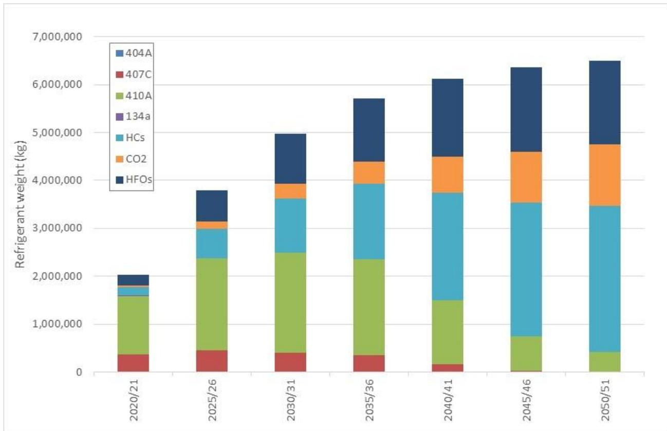
**Figure 21: Refrigerant Contained within Heat Pumps to 2050/51 (excluding AAHPs)**
