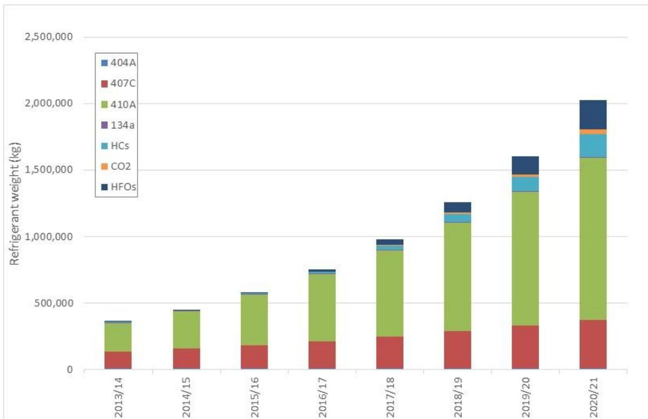
Figure 11: Projected Refrigerant Deployment to 2020/21 (excluding AAHPs)
