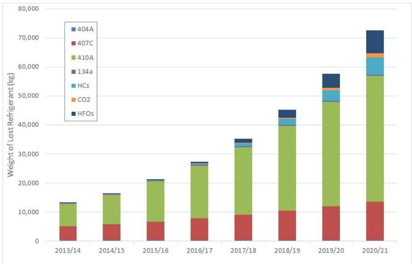
Figure 12: Operational Refrigerant Leakage to 2020/21 (excluding AAHPs)
