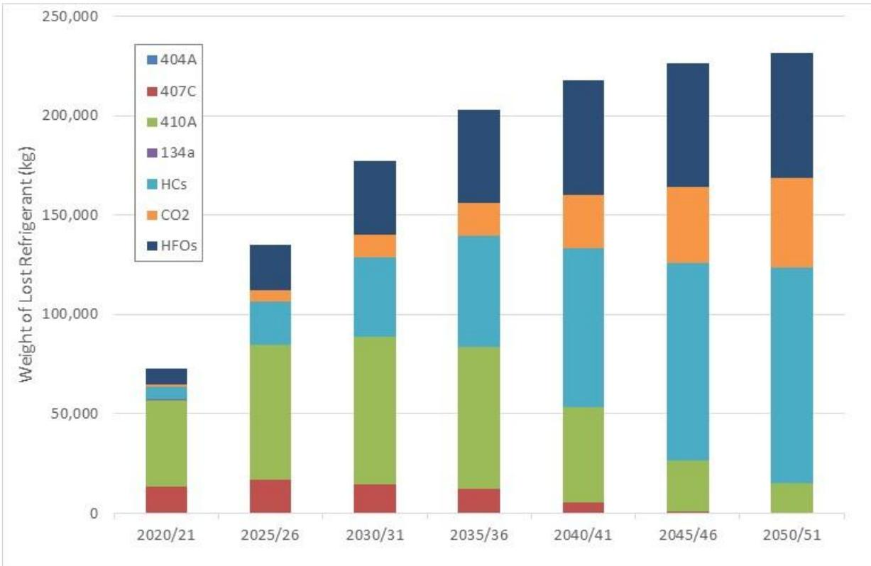
**Figure 22: Operational Refrigerant Leakage to 2050/51 (kg) (excluding AAHPs)**
