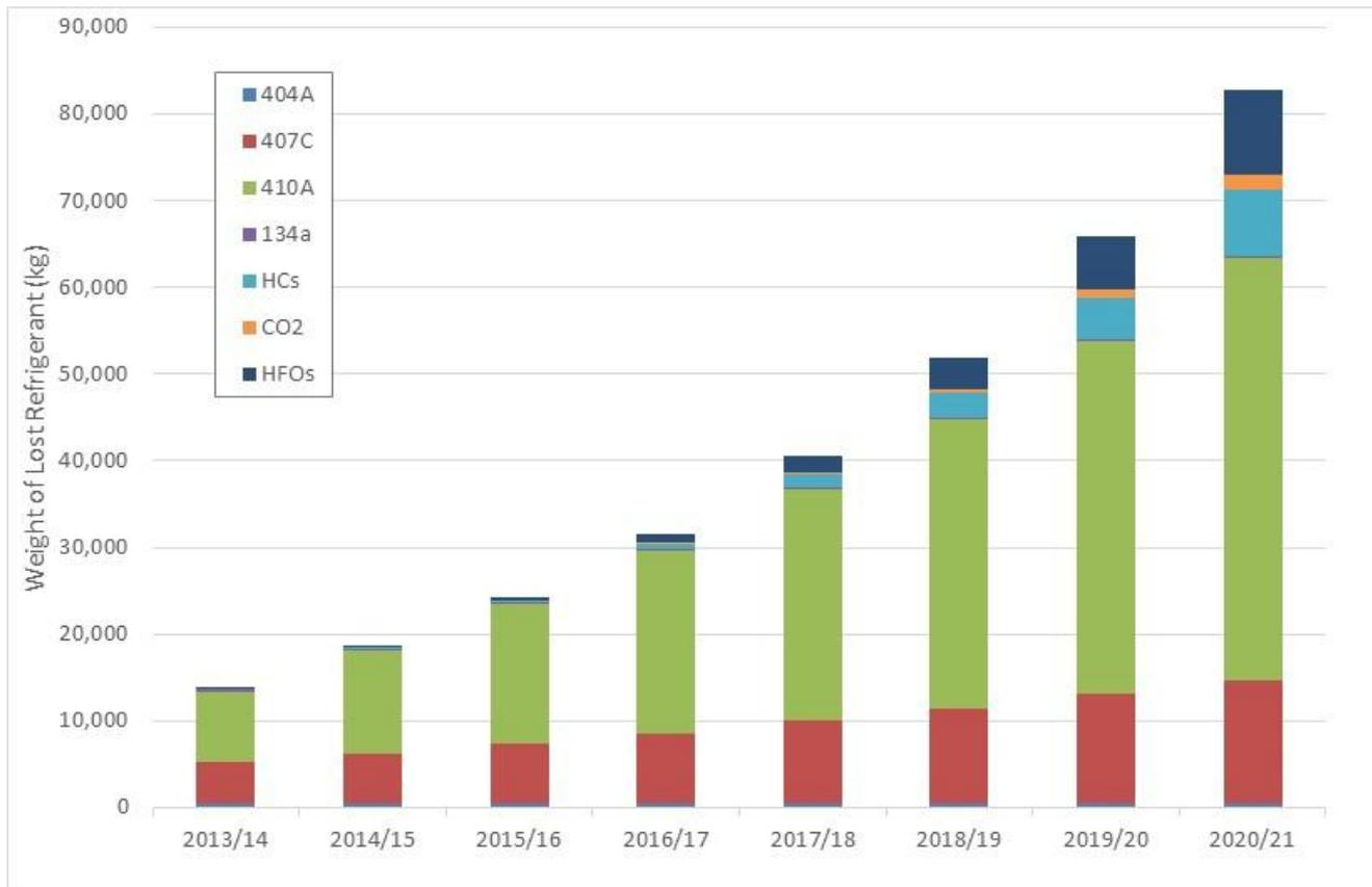
**Figure 13: Total Refrigerant Leakage to 2020/21 (excluding AAHPs)**
