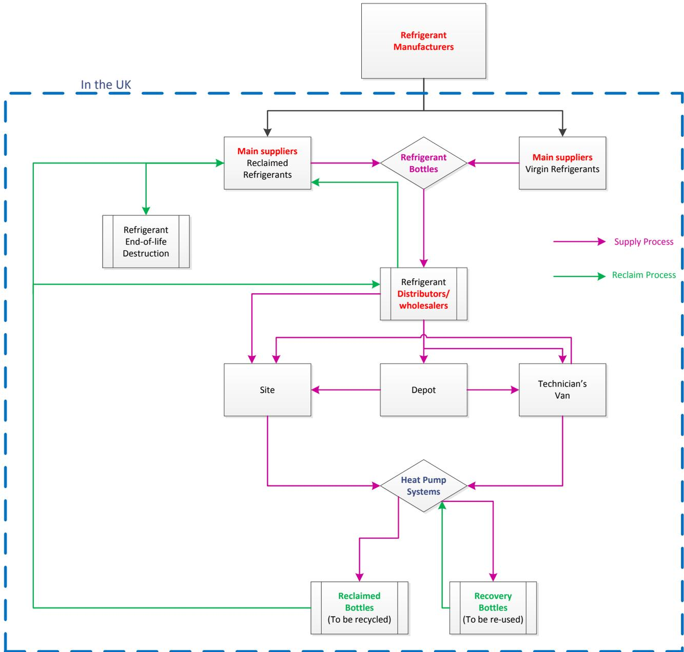
Figure 1: Schematic Representation of Refrigerant Supply Chain
