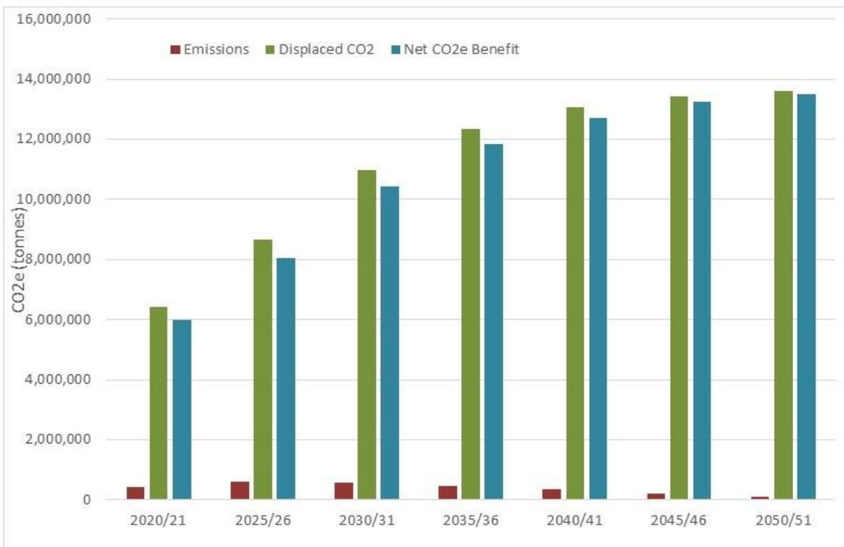
**Figure 27: CO<sub>2</sub>e Environmental Costs and Benefits of Heat Pumps to 2050/51 (tonnes CO<sub>2</sub>e) (including AAHPs)**
