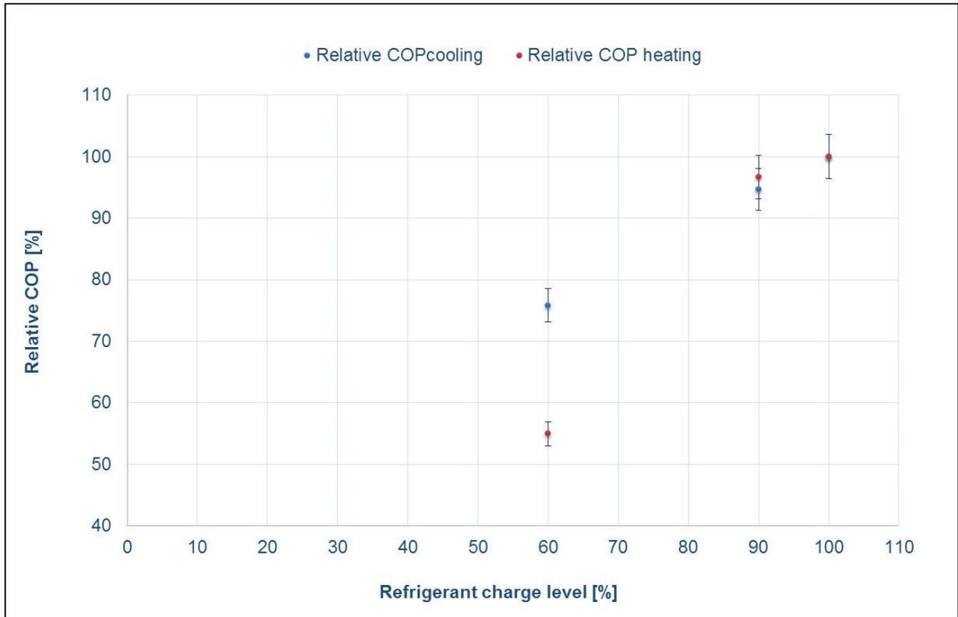
**Figure 3: Relative Change in Heating and Cooling COPs with Varying Refrigerant Charge**
