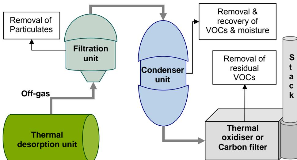
**Figure 4: Example of a TDU off-gas abatement system**
