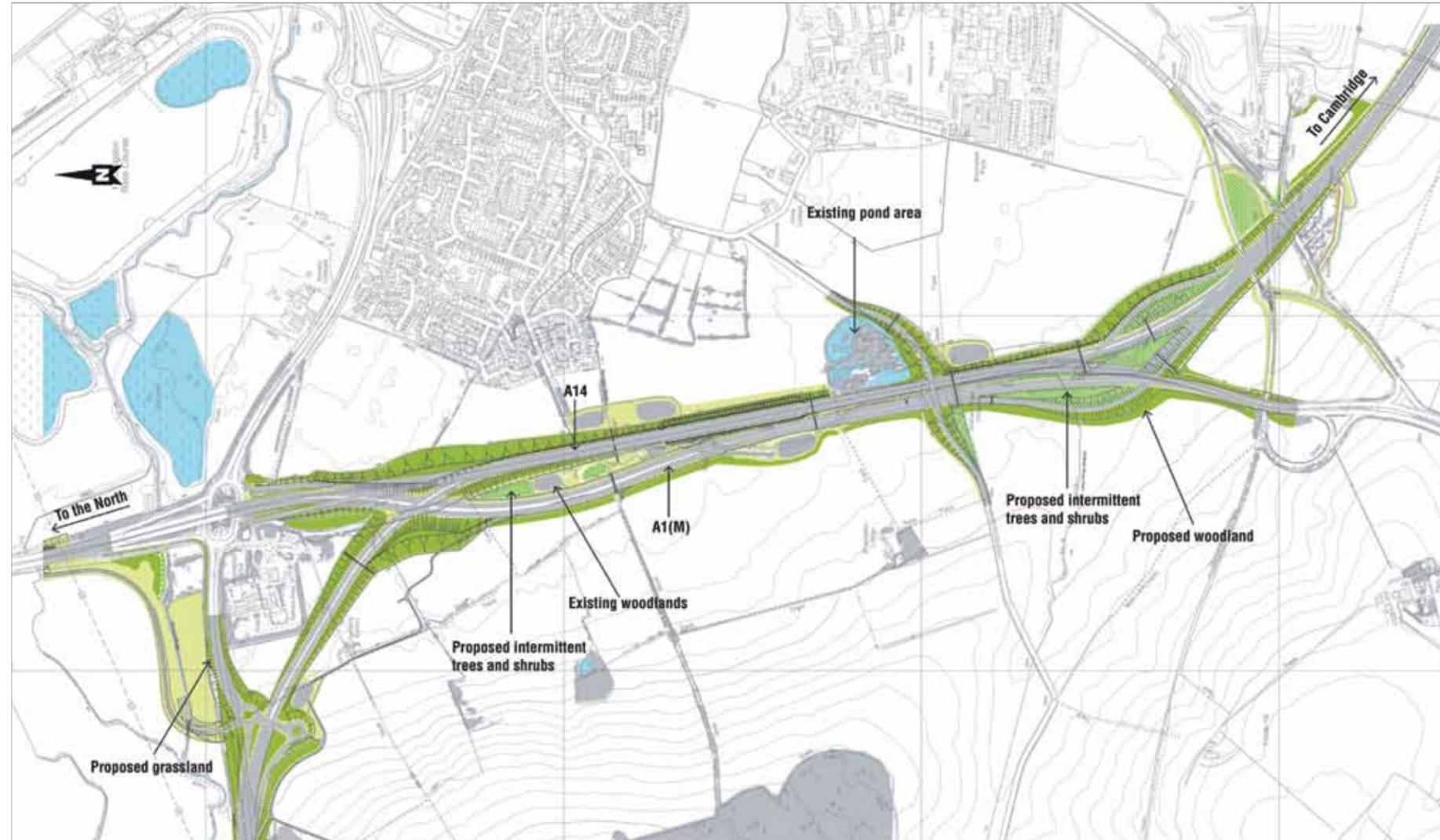
Figure 9: Widening of Alconbury to Brampton proposed layout
