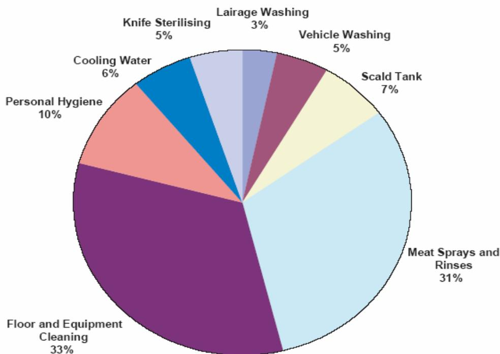
Figure 1 Typical water balance for areas in a pig abattoir
