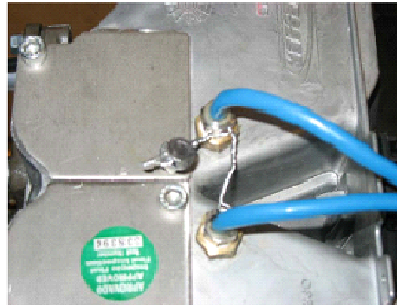
Figure 36.....Sealing – Temperature probes
