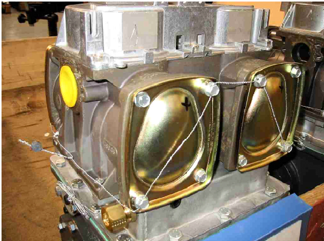
Figure 3 Wayne Global Hydraulics, meter sealing
