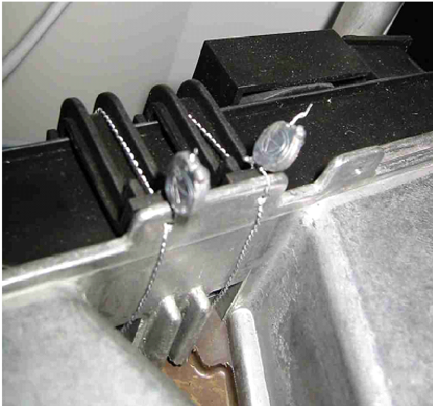
Figure 4 Sealing of Wayne Integrated Pulser (WIP)
