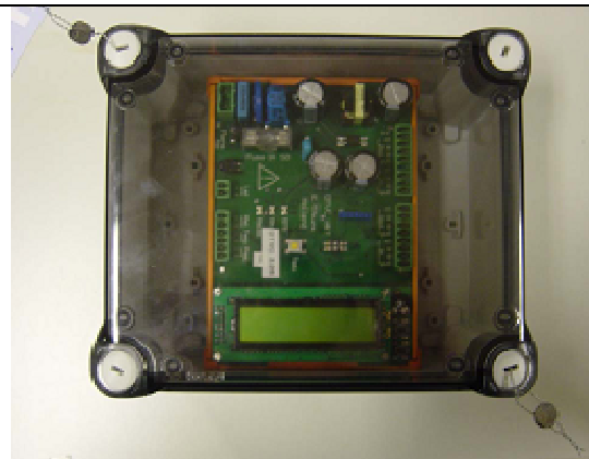
Figure 28 TVC unit sealing arrangement
